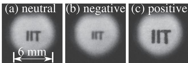
Fig. 2. Images taken through the lens for different positions of the screw. (a) Initially, the screw was turned to the position where the liquid-liquid interface was flat, that is, in the neutral state. The lens attains negative power (b) and positive power (c) when the screw is turned in and out, respectively. For these experiments, the lens was kept vertically such that the plane of aperture is parallel to the direction of gravity.
