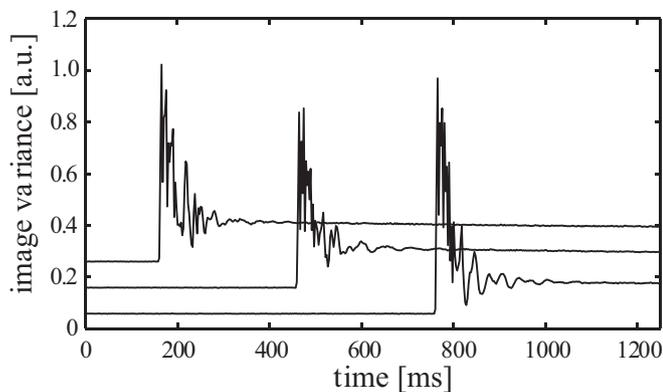
**Fig. 4.** Transient response of the liquid lens in three repeated experimental runs. The image variance shows oscillations upon sudden actuation. These oscillations diminish completely after 250 ms. The time response of the liquid lens is similar for all the experimental runs.
