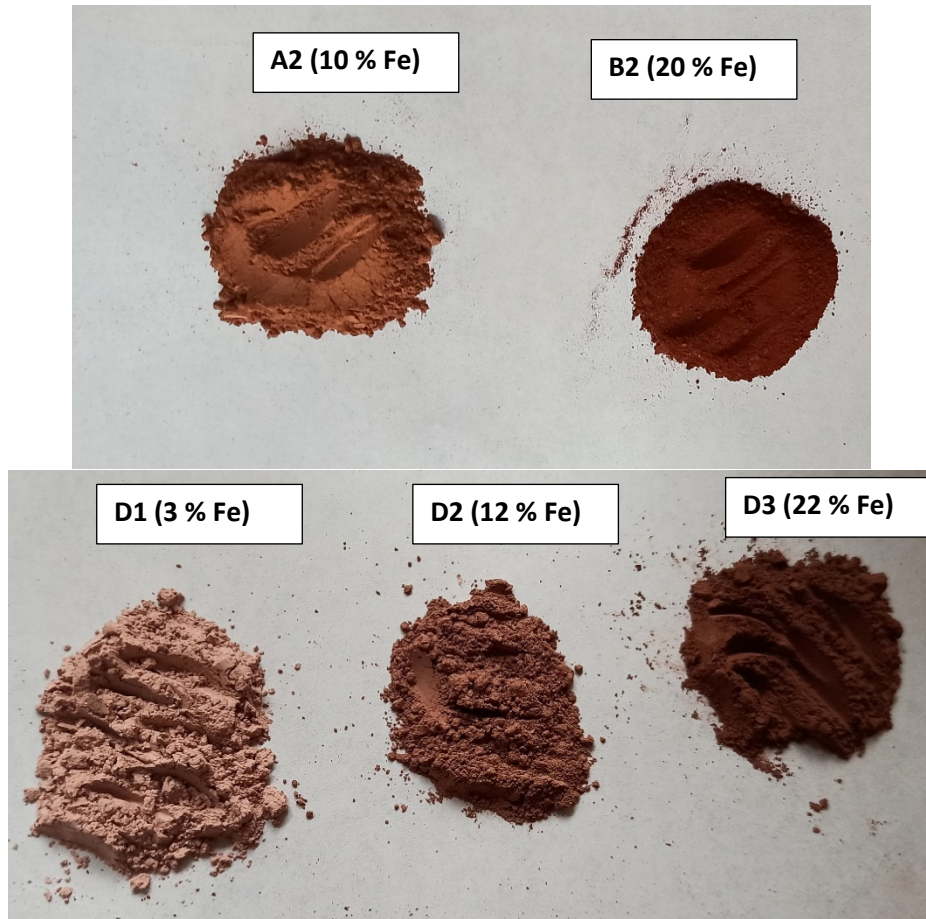
Figure 2: Clays with different iron contents
