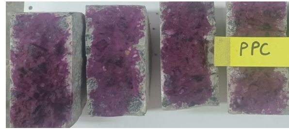
Fig. 4.2: Carbonation depth front in PPC
