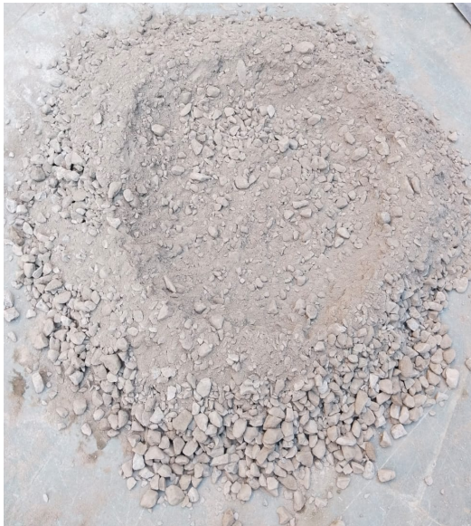
Fig. 1: Dry Mixing of mix design 1:1.5:3
