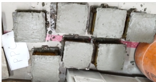
Fig.22: Cast cubes of PPC of mix design 1:1.5:3
