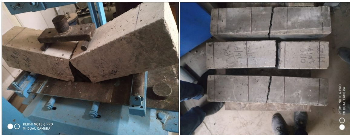
Figure 11 Flexure test in progress
