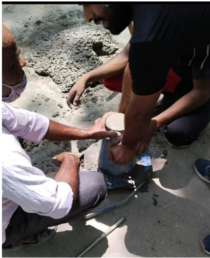
Fig.26: Slump measurement of Mix design 1:2:2
