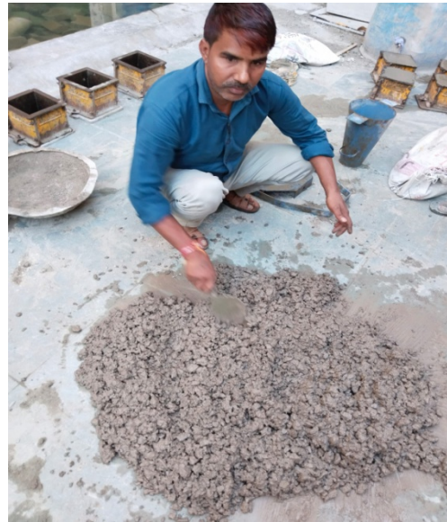
Fig. 19: Wet mixing and Trowel movement of mix design 1:1.5:3
