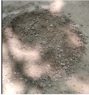
Fig.24: Dry Mix of Mix design 1:2:2
