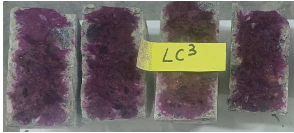
Fig. 4.1: Carbonation depth front in LC 3
