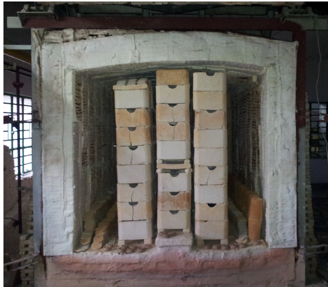
Figure 4.2: Saggars arranged in a shuttle kiln
