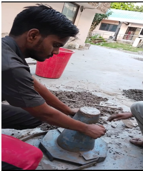
Fig. 20: Slump measurement of mix design 1:1.5:3
