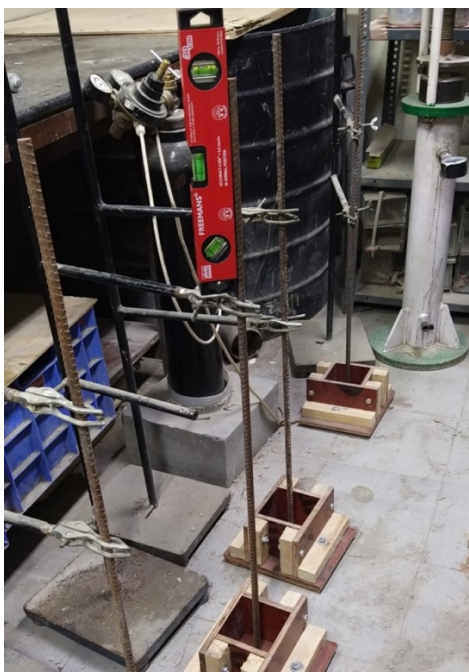
Figure 8 Casting of samples for pull-out test
