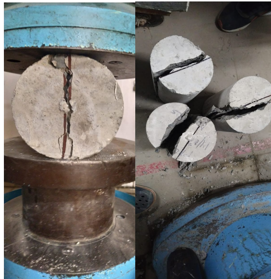
Figure 13 Split-tensile test in progress
