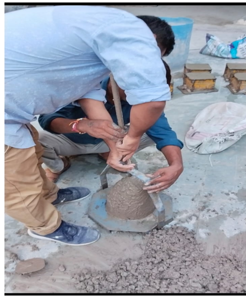
Fig. 21: Slump measurement of mix design 1:1.5:3
