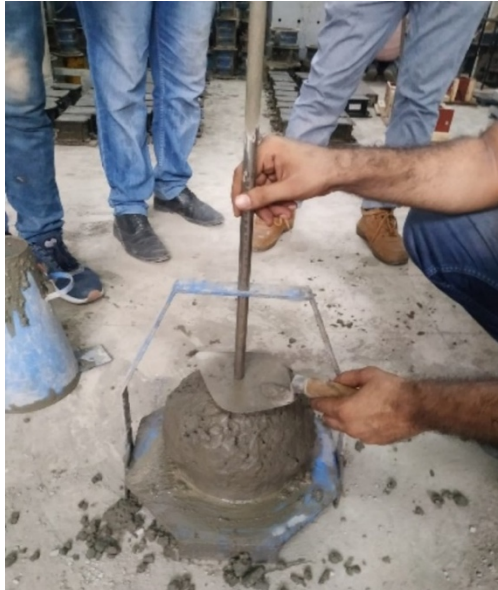
Figure 7 Slump test in progress
