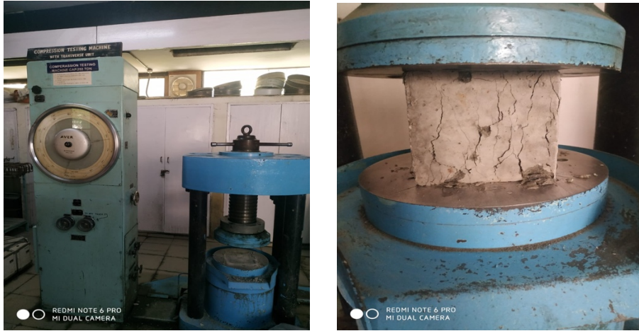
Figure 9 Test for compressive strength in progress
