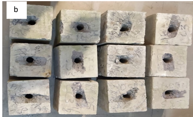
Figure 17 (a) Test arrangement for Pull-out strength, (b) failed specimens
