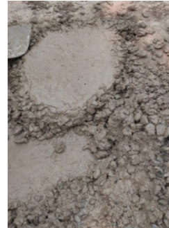
Fig.25: Dry Mix of Mix design 1:2:2
