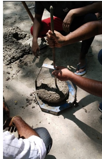
Fig. 27: Slump measurement of Mix design 1:2:2
