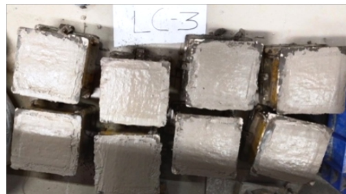
Fig.23: Cast cubes of LC3 of mix design 1:1.5:3
