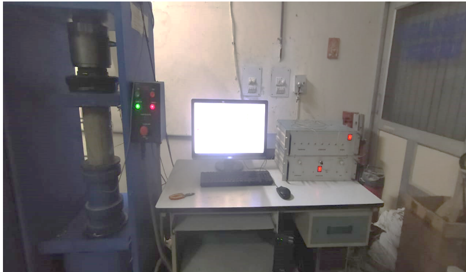
Figure 15 Arrangement of test for Modulus of elasticity using a data-logger
