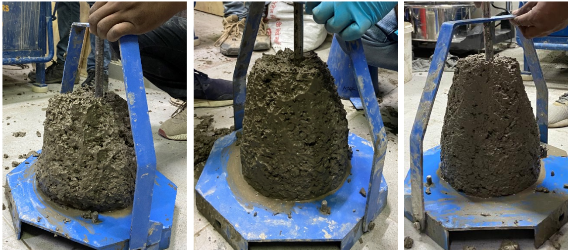
Figure 2: Concrete slump for mixes with c/a ratio of 0.68, 0.66 and 0.64
