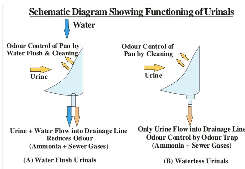
Figure 2. Schematic diagram showing functioning of urinals
