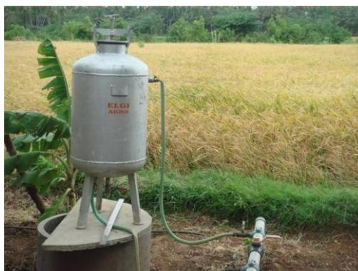
Figure20. Use of fertilisation tank for applying urine through drip irrigation (Photo: Prakash Kumar)
