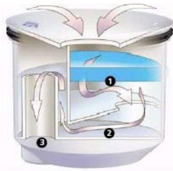
Figure 3. Sealant liquid based odour trap (source: waterwisetech.net)
