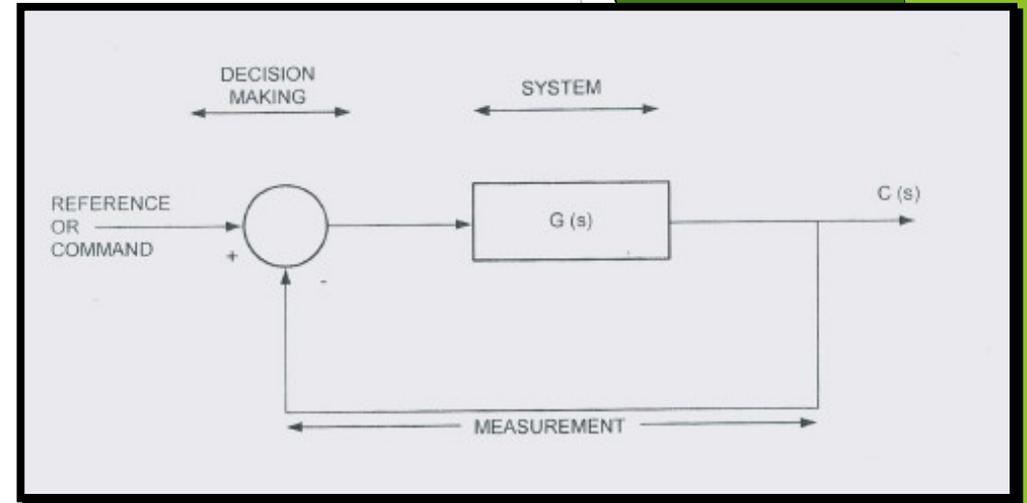
Fig 3: Closed Loop System
