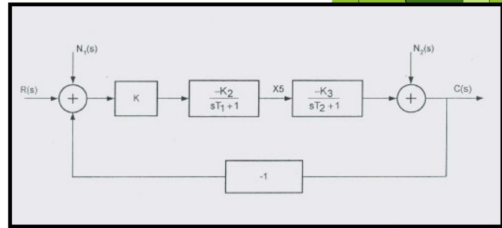
Fig 4: Block Diagram for Disturbance Rejection
