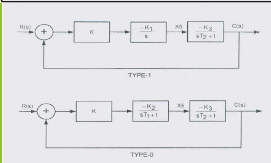
Table 2: Block Diagram of First & Second Order Closed Loop System
