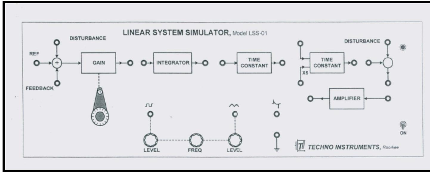
*Fig 1: Panel Diagram of Linear System Simulator*
