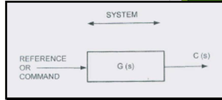
Fig 2: Open Loop System
