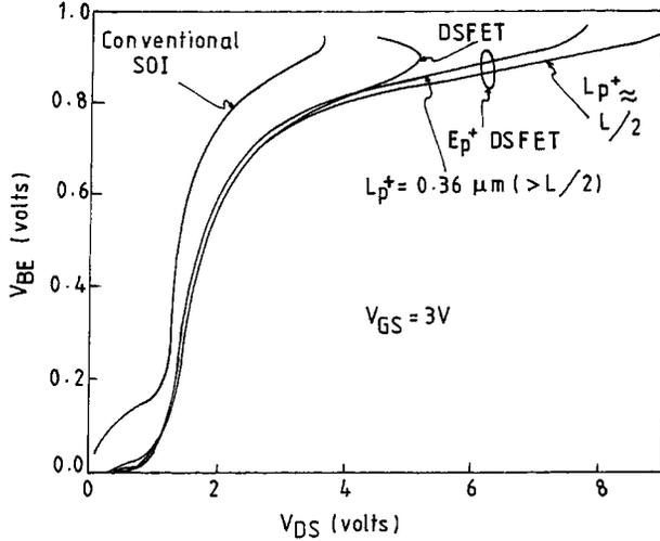
Fig. 3. Forward bias  $V_{BE}$  of the source-body junction versus the drain voltage  $V_{DS}$ .
