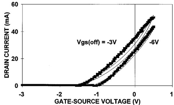
Fig. 1. Dynamic transfer characteristics, under a CW sinusoidal signal of 100 KHz and 3.5 V (peak to peak), measured approximately 1  $\mu\text{s}$  after the gate-source bias voltage was pulsed from either  $-3$  to  $-1.25$  or from  $-6$  to  $-1.25$  V. Shift in threshold voltage between the two cases indicates different amounts of trapped charges under different off-state gate-source voltages. (■) measured. (—) simulated.
