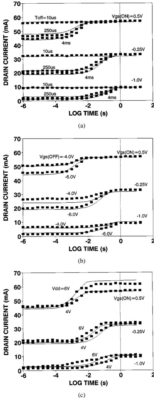
Fig. 3. (■) Measured and (—) simulated drain current transients showing their dependencies on on-state gate-source voltage as well as (a) off time, (b) off-state gate-source voltage, and (c) drain supply. When not varied, off time = 1 ms; off-state gate-source voltage =  $-6$  V; drain supply = 4 V.
