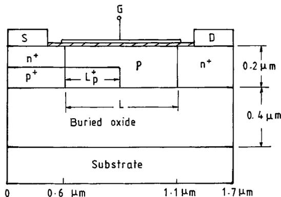
Fig. 1. Cross section of the extended  $p^+$  dual source SOI MOSFET where  $L$  is the channel length and  $L_{p^+}$  is the  $p^+$  region extended into the channel (Not drawn to scale).
