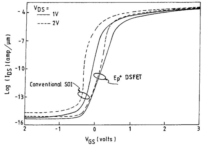
Fig. 6. Simulated  $I_{DS} - V_{GS}$  characteristics of conventional SOI MOSFET, DSFET and  $Ep^+$ DSFET.
