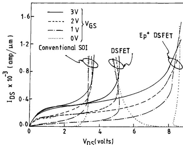
Fig. 2. Simulated  $I_{DS} - V_{DS}$  characteristics of conventional SOI MOSFET, DSFET and  $Ep^+$  DSFET.
