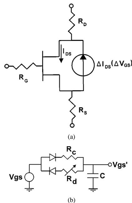
Fig. 2. Circuit model implemented in SPICE. (a) Parasitic current source  $\Delta I_{DS}$  is modeled as another MESFET and is used to mimic the threshold voltage shift. (b) Nonlinear RC timing circuit is used to drive the parasitic current source. The voltage dependence of the detrapping time constant  $\tau_D$  ( $V_{GS}$ ,  $V_{DS}$ ) is modeled by using a variable resistor.
