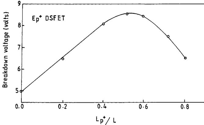
Fig. 4. Breakdown voltage versus  $L_{p^+}/L$  for the  $Ep^+$ DSFET with channel length  $L = 0.5 \mu\text{m}$ .
