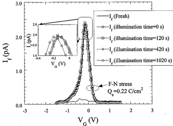
Fig. 2. Measured forward gated-diode current versus gate voltage from one n-MOSFET sample. The gate oxide area was  $3 \mu\text{m}^2$ . For the selected illumination time following  $Q_e$  of  $0.22 \text{ C/cm}^2$ , the filling scheme was interrupted and the test setup was switched to the forward gated-diode configuration. The  $I$ - $V$  near the current peak is magnified for clear viewing.
