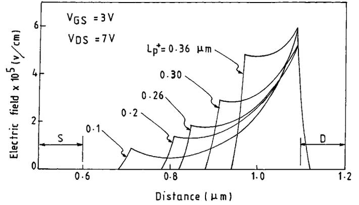
Fig. 5. Electric field along the  $x$ -axis in the body at a depth of  $0.14 \mu\text{m}$  from the  $\text{Si}/\text{SiO}_2$  interface for different values of  $L_{p^+}$ .
