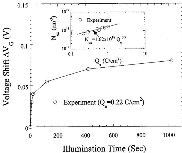
Fig. 3. Gate voltage shift versus illumination time corresponding to Fig. 2. The inset shows the estimated trap density  $N_{ox}$  versus  $Q_e$  from seven n-MOSFET samples. Each sample represents a specific  $Q_e$ . A power law relation is drawn by best fitting data points.
