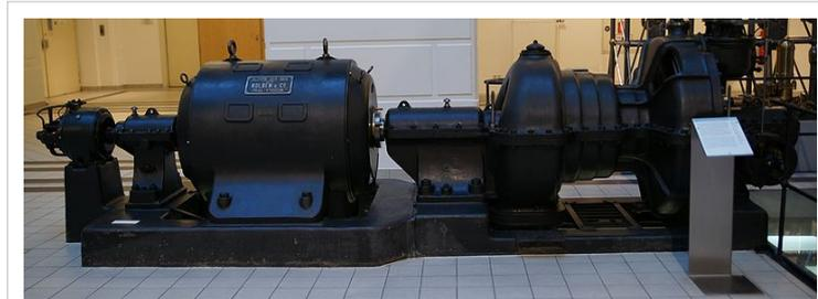
A small industrial steam turbine (right) directly linked to a generator (left). This turbine generator set of 1910 produced 250 kW of electrical power.
