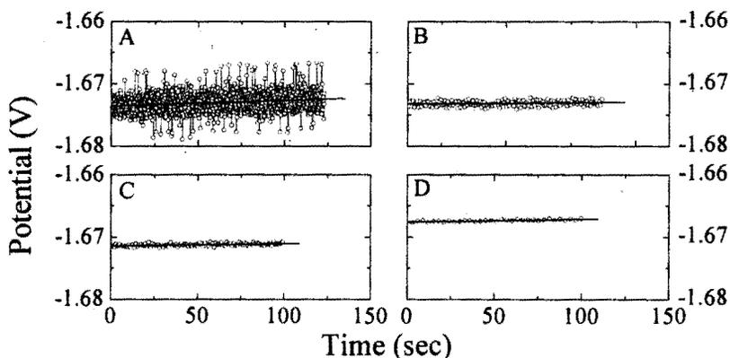
Fig. 1: Standardization of signal averaging period for the ADC card in standard buffer of pH 4. [A] Averaging time of 100 m sec (SD 17.1 mV); [B] 500 m sec (SD 4.45 mV); [C] 1000 m sec (SD 2.19 mV) and [D] 2000 m sec (SD 1.09 mV).
