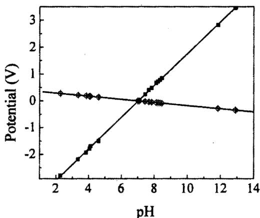
Fig. 2: Calibration of the computer controlled pH meter with respect to commercial analog pH meter. Straight-line fit for [o] commercial pH meter, ( $Y = 0.40913 - 0.05845 \times X$ ); [+ ] 1st op-amp output, ( $Y = 0.40839 - 0.05832 \times X$ ) and [■] 2nd op-amp output ( $Y = -4.1544 + 0.59082 \times X$ ) of the fabricated instrument.
