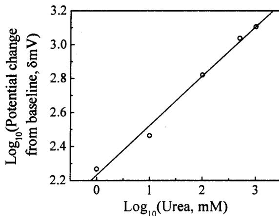
Fig. 5: The calibration curve for the biosensor at 180 sec response time (derived and plotted from Fig. 4).  $R^2 = 0.9951$ .
