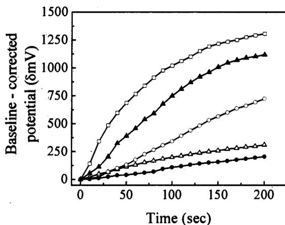
Fig. 4: The biosensor response curves for (●) 1 mM, (Δ) 10 mM, (○) 100 mM, (▲) 500 mM and (□) 1 M urea.
