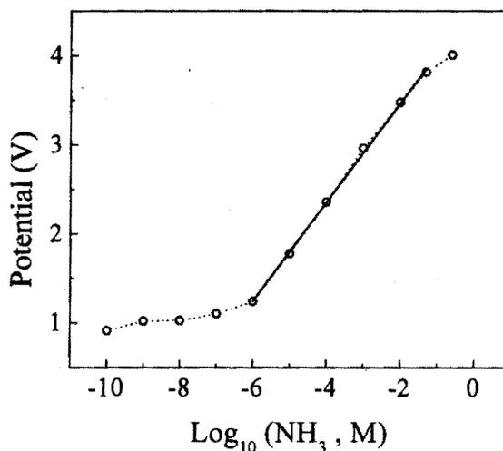
Fig. 3: Nernstian behaviour of pH meter with respect to different concentrations of  $\text{NH}_3$  (dotted line). Straight-line fit at central portion of curve represents  $Y = 0.55533 \times X + 4.57511$ ,  $\text{Chi}^2 = 0.00121$ ,  $R^2 = 0.99902$ .
