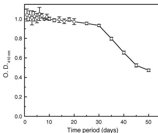
Fig. 5. Storage stability of the immobilized microbial enzyme on glass fiber filter paper. A concentration of 50 µM methyl parathion was used for the study.
