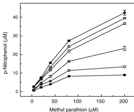
Fig. 3. Effect of loading different cell densities for immobilization: (■) normal harvested cell density; (○) 2.5-fold; (△) 5-fold; (◇) 10-fold; (◆) 20-fold; (□) 25-fold increase of cell density.
