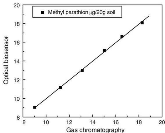
Fig. 6. Correlation of the optical biosensor measurement with the gas chromatography for methyl parathion spiked sample. (■) Methyl parathion with concentrations of 10, 12, 14, 16, 18 and 20 µg per 20 g of soil.
