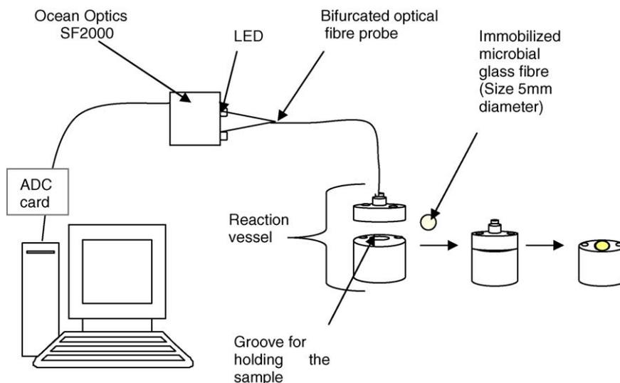
Fig. 1. Schematic diagram of operating system of optical fiber biosensor and reaction vessel.
