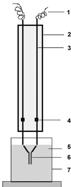
**Fig. 1.** Schematic diagram of Pt-twin wire electrode. The components shown are: (1) copper wire contacts connecting to bipotentiostat, (2) glass body filled with epoxy, (3) copper wire, (4) solder (contact), (5) PSS–PAni or other buffer solutions, (6) Pt wires converging at a gap of 100  $\mu\text{m}$  (which is the site of formation of dark green PSS–PAni) and (7) glass beaker of 5 ml capacity.
