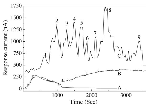
**Fig. 3.** Electropherograms of: (A) 25-mer ssDNA (poly-A); (B) 25 bp dsDNA (polyA-T); (C) 1.5 kb DNA ladder detected using amperometric method. Separation channel length = 2 cm, separation voltage: 100 V, detection voltage: 0.7 V, buffer solution: 1X PBS, pH 7.4. Peaks: (1:100, 2:200, 3:300, 4:400, 5:500, 6:600, 7:800 and 9:1500 bp DNA).
