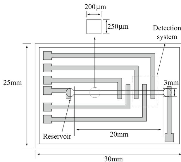
Fig. 2. Schematic diagram of CE-AD microchip.
