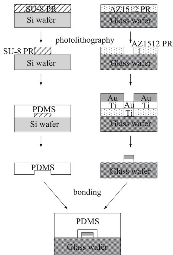
Fig. 1. Microchip fabrication process.
