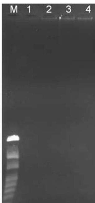
**Fig. 4.** Gel-doc showing DNA extracted from lysis of MCF-10A cell line on the chip. Lanes: M = 1.5 kb marker (6  $\mu$ L loading); 1 = 0 V; 2 = 2 V; 3 = 5 V; 4 = 10 V (lanes 1–4 = 20  $\mu$ L sample loading). A minimum potential of 2 V was required for lysis, whereas 5 V was ideal for effective genomic DNA extraction. The genomic DNA bands can be seen just below loading wells, whose respective concentrations were 0, 0.4, 0.7 and 1.0  $\mu$ g/ml for 0–10 V treatment.
