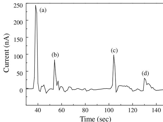
Fig. 4. Electropherogram of a mixture of 1 mM each of (a) BPA, (b) butylphenol, (c) phenylphenol, and (d) nonylphenol with PB/ITO electrode.
