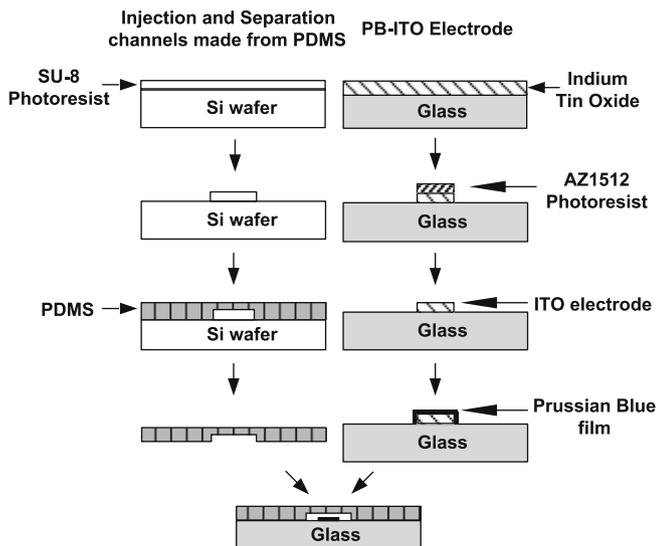
Fig. 1. Process flow for the fabrication of the CE/ECD microchip.
