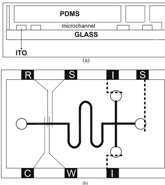
Fig. 2. Configuration of PDMS mold containing microchannels: side (a) and top view (b).
