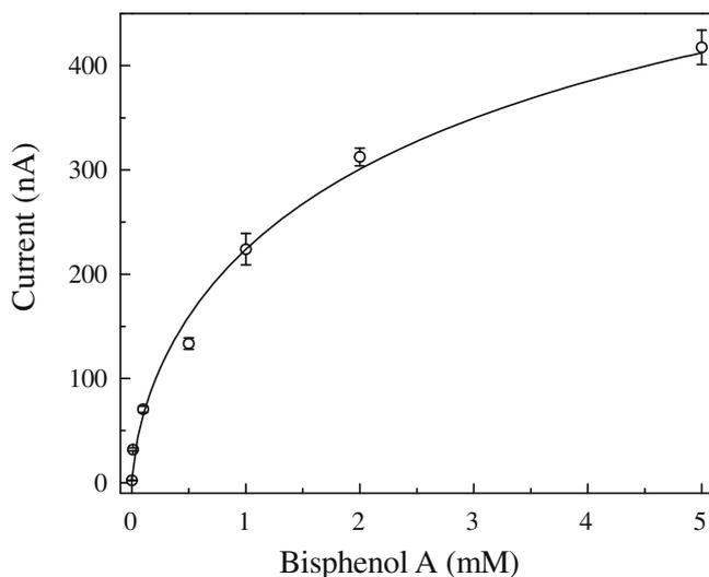
Fig. 3. Concentration dependent response current for analyte bisphenol A. Error bars represent standard deviation of triplicate measurements.
