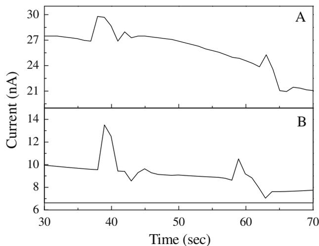
Fig. 5. Electropherogram of Styrofoam water extract (A) and of Styrofoam water extract spiked with 1  $\mu\text{M}$  BPA and butylphenol (B) using PB/ITO electrode.
