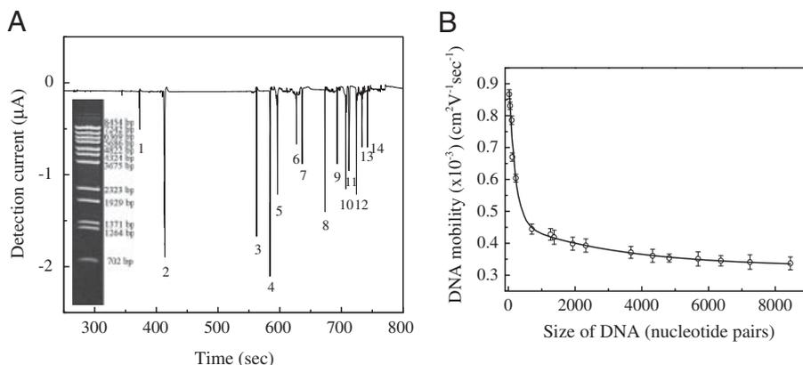
**Figure 5.** (A) Electropherogram of CE-AD separation of commercial DNA ladder (migration time for 14 fragments shown as numbers) at separation voltage of 100 V dc and detection voltage of 0.82 V (inset shows gel doc of DNA ladder on a 7% agarose gel); (B) DNA mobility coefficient for each DNA fragment calculated from Eq. (1). The converged curve fit used exponential decay-3 equation model from Origin™ software (version 8).
