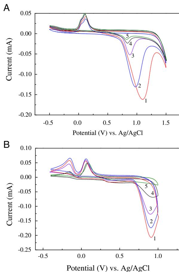
**Figure 2.** CV of nucleosides at different concentrations (1: 1 mM, 2: 100  $\mu$ M, 3: 10  $\mu$ M, 4: 1  $\mu$ M and 5: 100 nM) using conventional disc electrodes of 2 mm diameter and reaction vessel from CH Instruments: (A) adenosine and (B) guanosine in 100 mM NaOH; scan rate: 100 mV/s.
