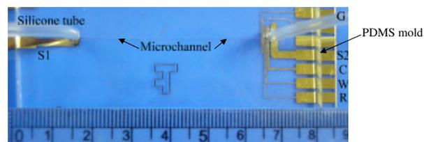
**Figure 1.** Image of CE-AD microchip showing microchannel engraved in PDMS mold, sample reservoirs, silicon tubes carrying sample and NaOH solution into the microchannel, gold microelectrodes (W, working; C, counter; R, reference; G, decoupler ground electrodes; S1 and S2, separation electrodes) and contact pads.
