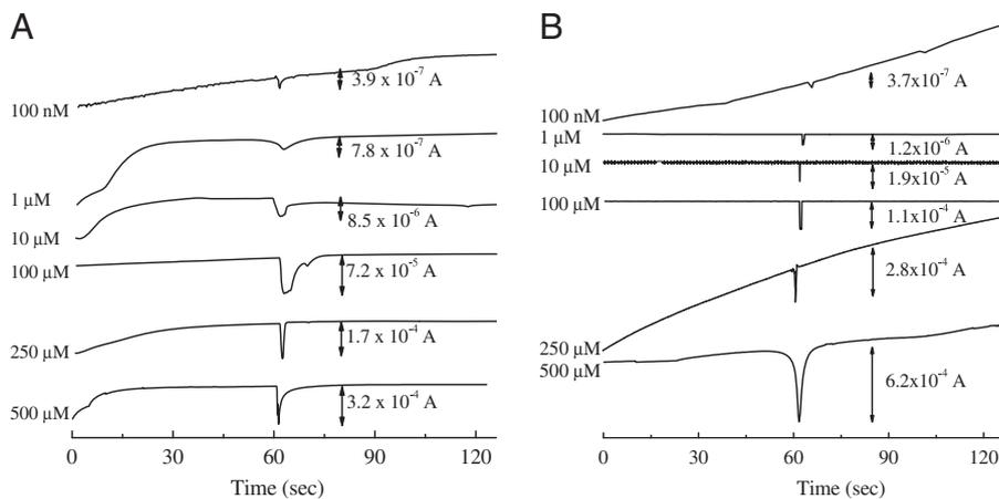
**Figure 3.** Electropherograms of (A) adenosine and (B) guanosine at 100 nM, 1  $\mu$ M, 10  $\mu$ M, 100  $\mu$ M, 250  $\mu$ M and 500  $\mu$ M concentrations at separation voltage: 100 V dc, detection voltage: 0.92 and 0.82 V (respectively).
