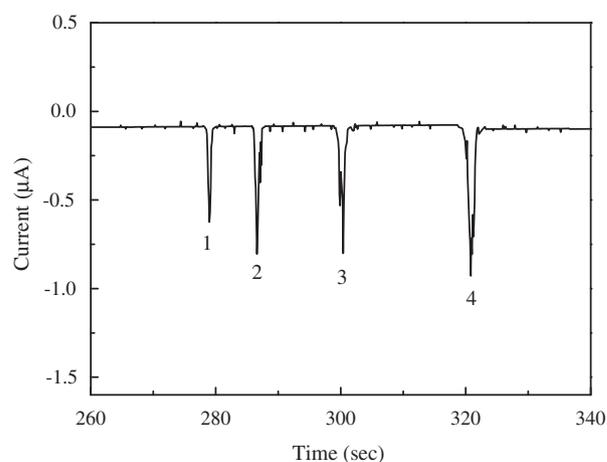
**Figure 4.** Electropherogram of a mixture containing 500 pmol each of (1) 25-mer polyA ssDNA; (2) 25-, (3) 50 and (4) 100-mer poly AT dsDNA at separation voltage 100 V dc and detection voltage 0.92 V.
