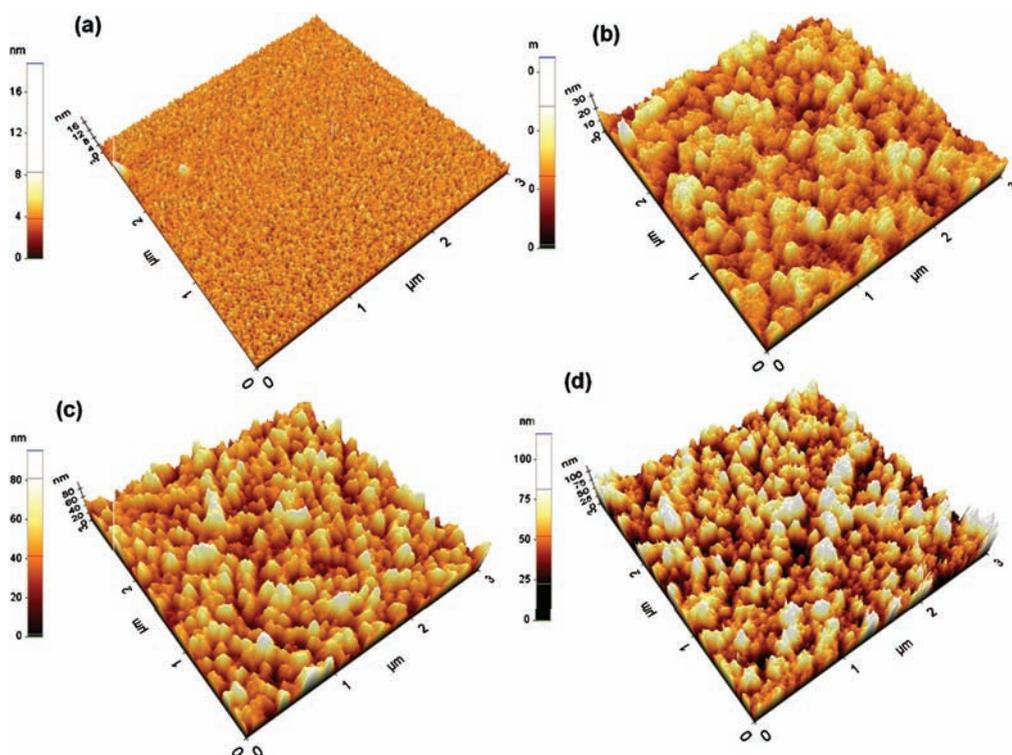
**Fig. 5.** AFM images of the bare gold substrate (a), after the immobilization of 1,6-hexanedithiol (b), after modified by gold nanoparticle on 1,6-hexanedithiol linker (c), and finally after the deposition of  $\beta$ -amyloid(1-42) protein.
