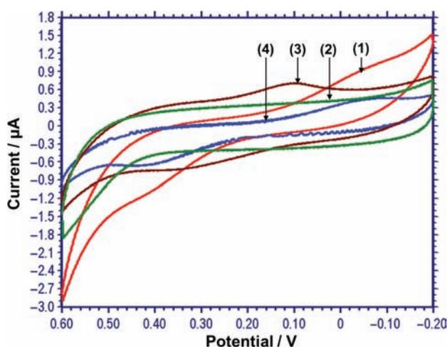
**Fig. 4.** Cyclic voltammogram of: (1) bare gold electrode; (2) 1,6-hexanedithiol modified electrode; (3) 1,6-hexanedithiol/Au-colloid modified electrode; (4) after deposition of  $A\beta$ (1-42) peptide. Solution composition: 0.1 M  $Na_2HPO_4$ - $NaH_2PO_4$  and 1.0 mM  $K_3[Fe(CN)_6]/K_4[Fe(CN)_6]$  with scan rate 0.05  $Vs^{-1}$ .
