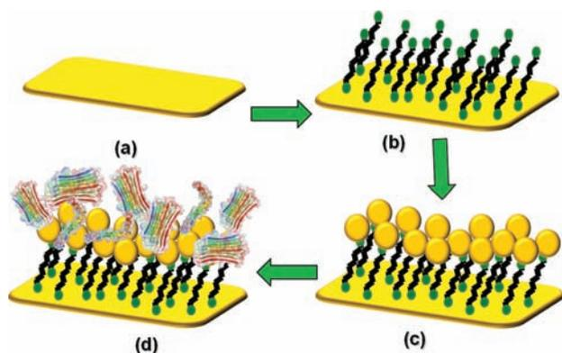
**Fig. 3.** Model of surface modification on gold electrode. a–b: self-assembly of 1,6 hexanedithiol as cross-linkers, c: 1,6-hexanedithiol/Au-colloid modification, d: after deposition of  $A\beta(1-42)$  peptide.
