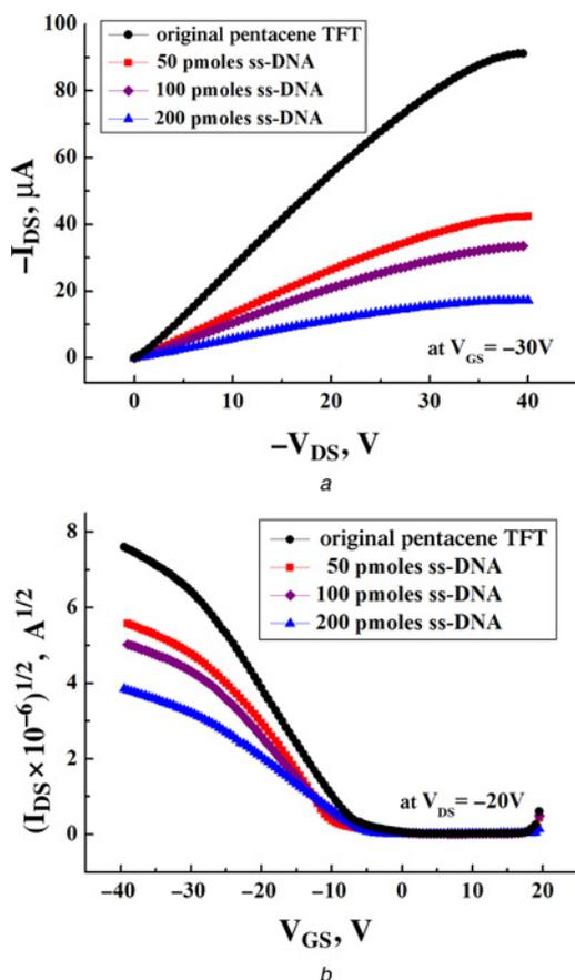
**Figure 3** Pentacene FETs with 50, 100 and 200 pmol DNA immobilised on pentacene surface
