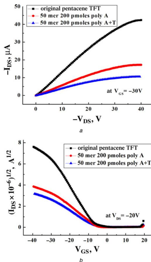
**Figure 2** Performance of the pentacene FETs with DNA immobilised on pentacene surface
