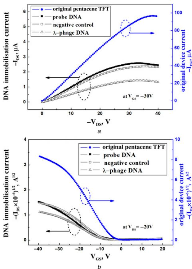
**Figure 4** Performance of the pentacene FETs with single-stranded 20-mer probe immobilised on pentacene surface and on hybridisation of  $\lambda$ -phage DNA
