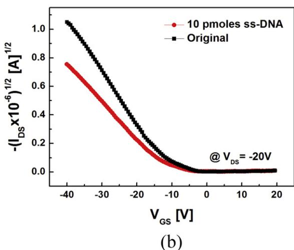
Fig. 5. Performance of the pentacene TFTs with immobilized DNA on pentacene surface: (a) output characteristics and (b) transfer characteristics of two pentacene TFTs (original, ss-DNA).
