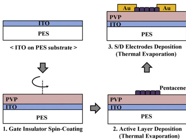
Fig. 1. Fabrication procedure of the pentacene TFTs.
