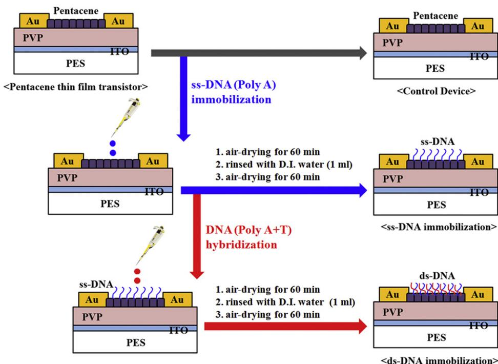
Fig. 2. Schematics showing the DNA immobilization and hybridization on the OTFTs.
