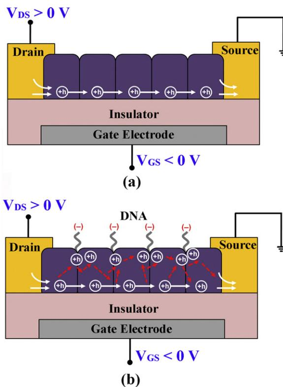
Fig. 4. DNA sensing mechanism on the pentacene TFTs. The device characteristics of an OTFT (a) w/o DNA immobilization and (b) w/DNA immobilization.
