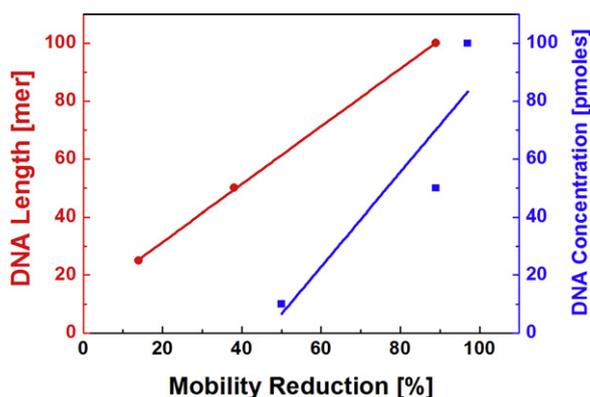
Fig. 6. Reduction ratio of field-effect mobility for the pentacene TFTs with immobilized ss-DNA, with respect to original device, as a function of DNA length and DNA concentration.
