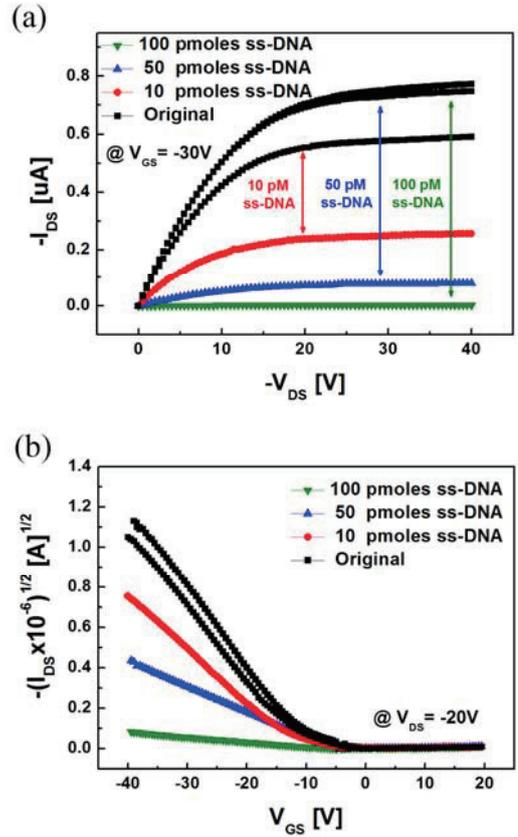
Figure 4. (a) Output characteristics and (b) transfer characteristics of a pentacene TFTs with 10, 50 and 100 pmoles DNA immobilized on pentacene surface.
