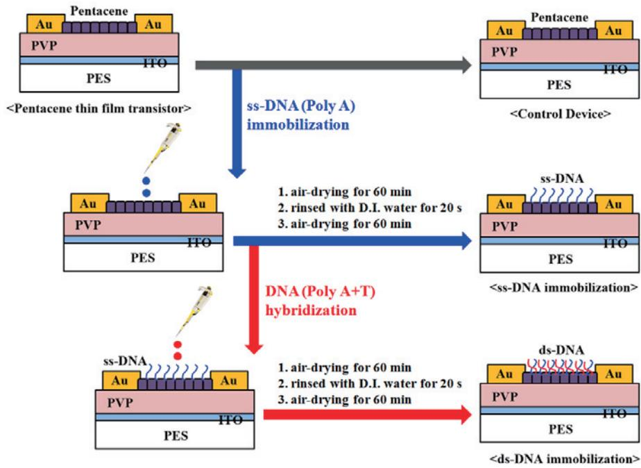
Figure 1. Scheme showing the DNA immobilization and hybridization in the OTFTs.
