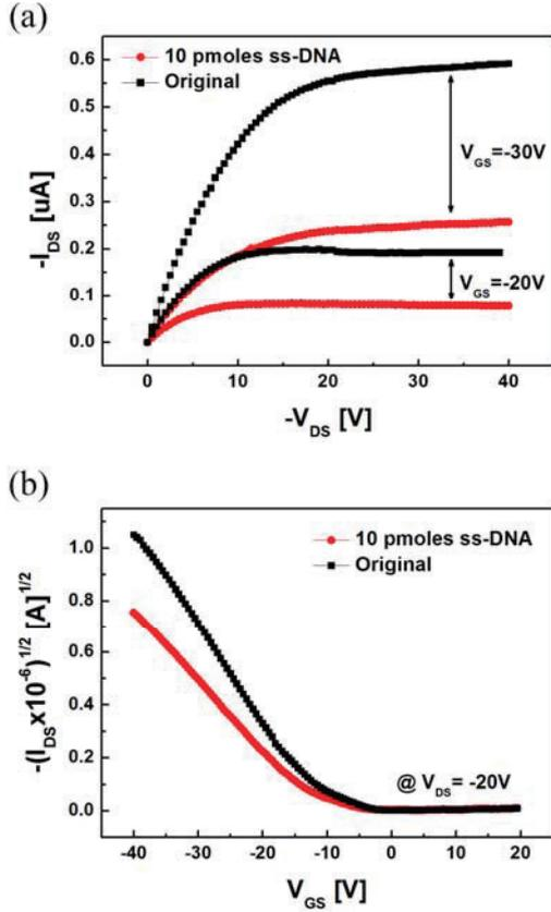
Figure 3. Performance of the pentacene TFTs with DNA immobilized on pentacene surface for 60 min: (a) output characteristics of two pentacene TFTs (original, ss-DNA), (b) transfer characteristics of two pentacene TFTs (original, ss-DNA).
