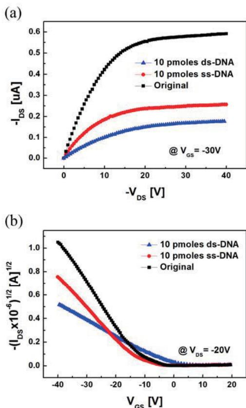
Figure 5. Performance of the pentacene TFTs with DNA immobilized on pentacene surface for 30 min. (a) output characteristics of three pentacene TFTs (original, ss-DNA, ds-DNA); (b) transfer characteristics of three pentacene TFTs (original, ss-DNA, ds-DNA).
