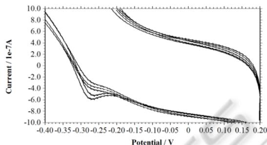
Figure 3: CV showing peaks for different concentrations of MB-DNA complex in 200 mM KCl, Scan rate: 0.1 V/s.
