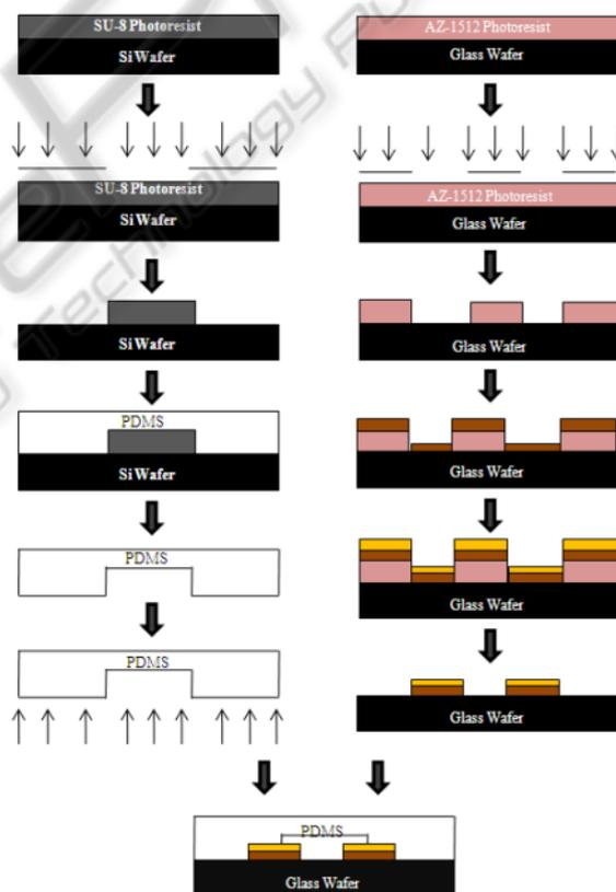
Figure 1: Fabrication of CE-AD device.
