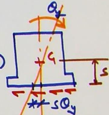
Rotation  $\rightarrow \phi_y \ddot{\theta}_y + K_{Qy} \theta_y = M(t) + \underbrace{K_{Tx} (x - s\theta_y) s}_{\text{Moment of shear stress}} + Mg s \theta_y$
