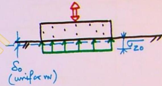
$C_\tau$  = Coefficient of elastic uniform shear
