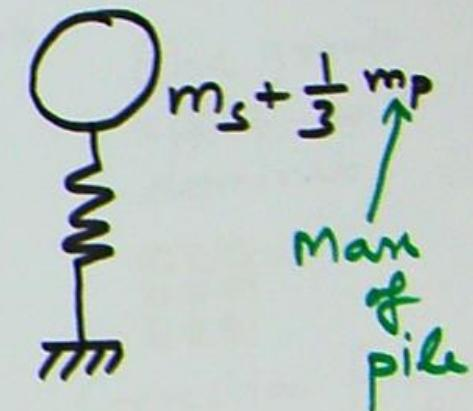
Idealize pile as a rigid bar undergoing axial vibrations
