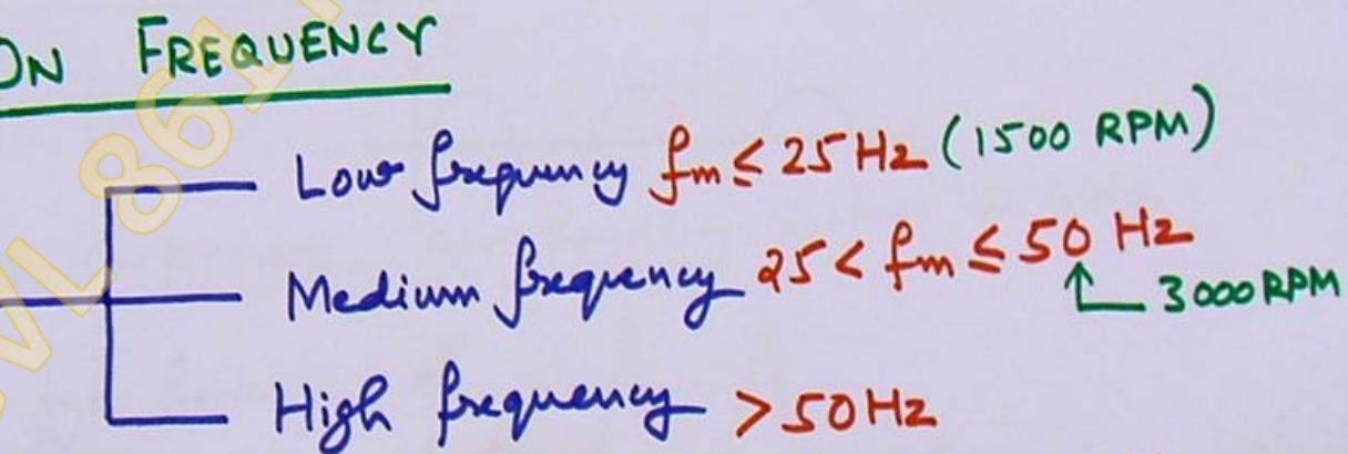
Low : Eg: Compressors, pumps.  $f_m < f_N$ . Block type fdm. resting on soil directly.
