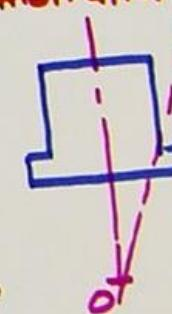
DOF positioned at combined CG "G" of block + Base + M/c.
