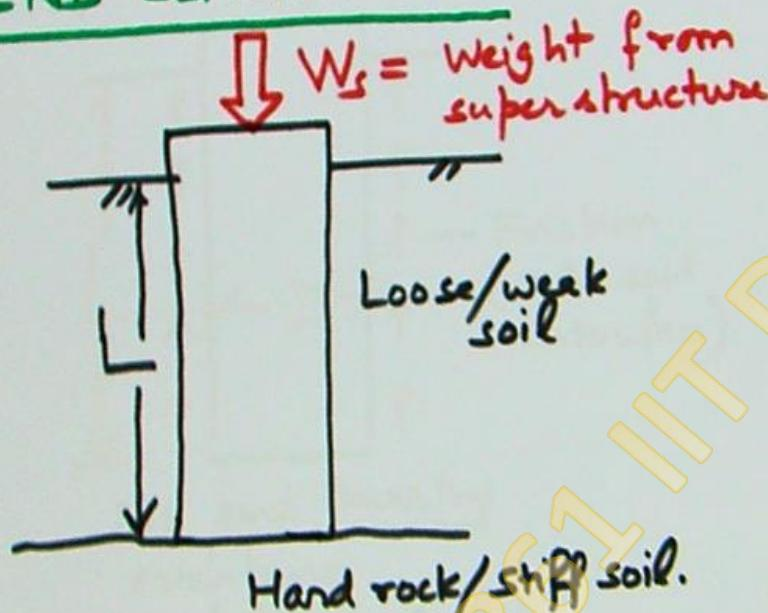
$$\text{Lumped mass} = \frac{W_s}{g} = \frac{N}{g} = m_s \text{ kg}$$
