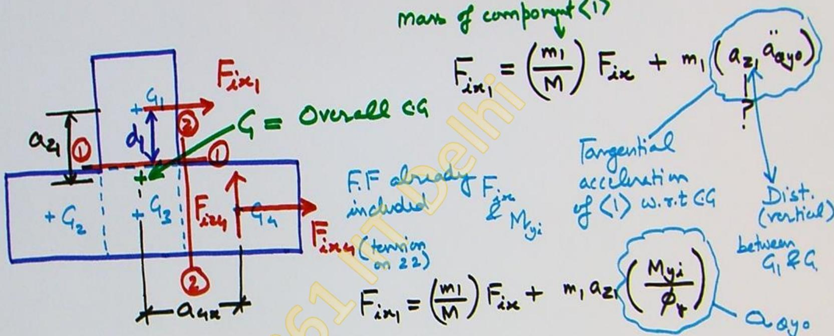
Bending moment acting on plane 11 =  $F_{ix1} \times d_1$
