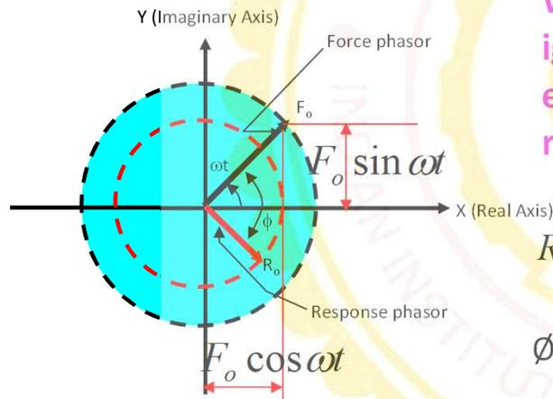
$$R = R_o \cos(\omega t - \phi) + jR_o \sin(\omega t - \phi) = u_o e^{j(\omega t - \phi)}$$
