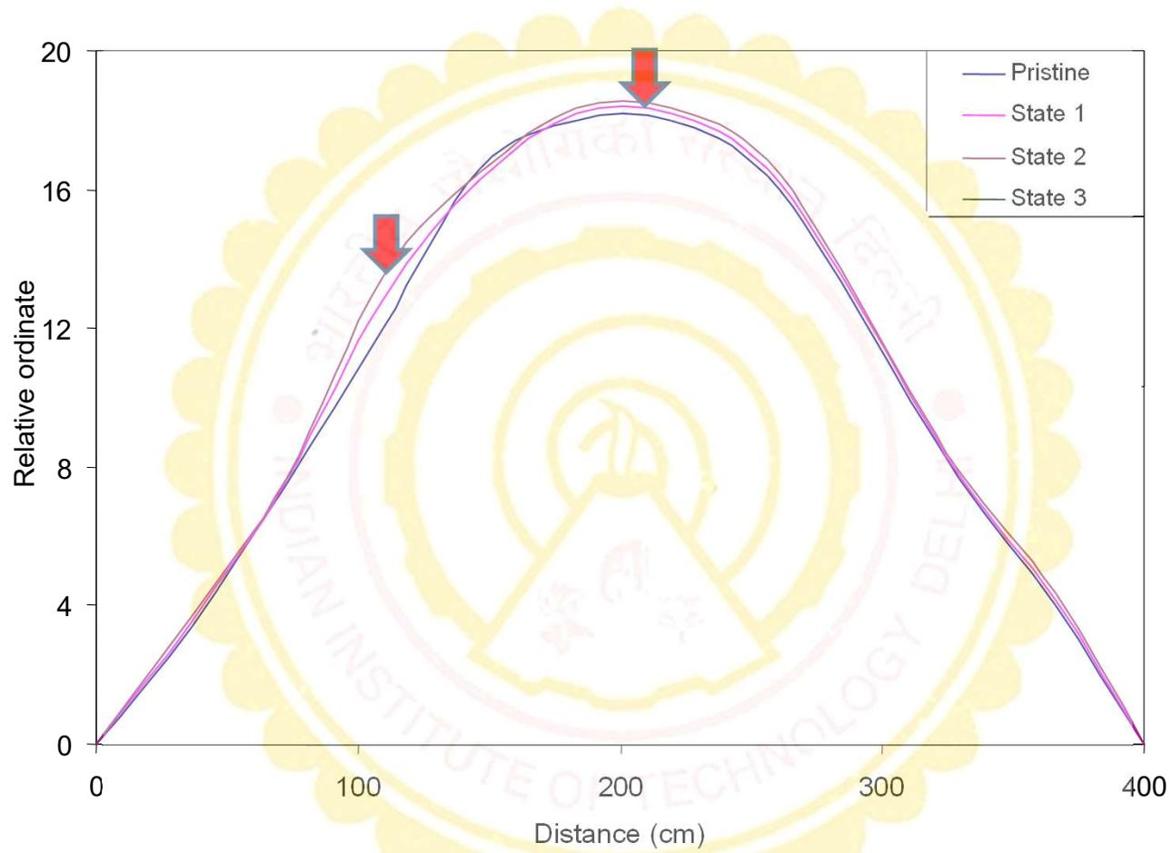
**Curvature mode shape from piezo patches**
