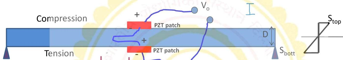
*Strain or curvature mode shape*
