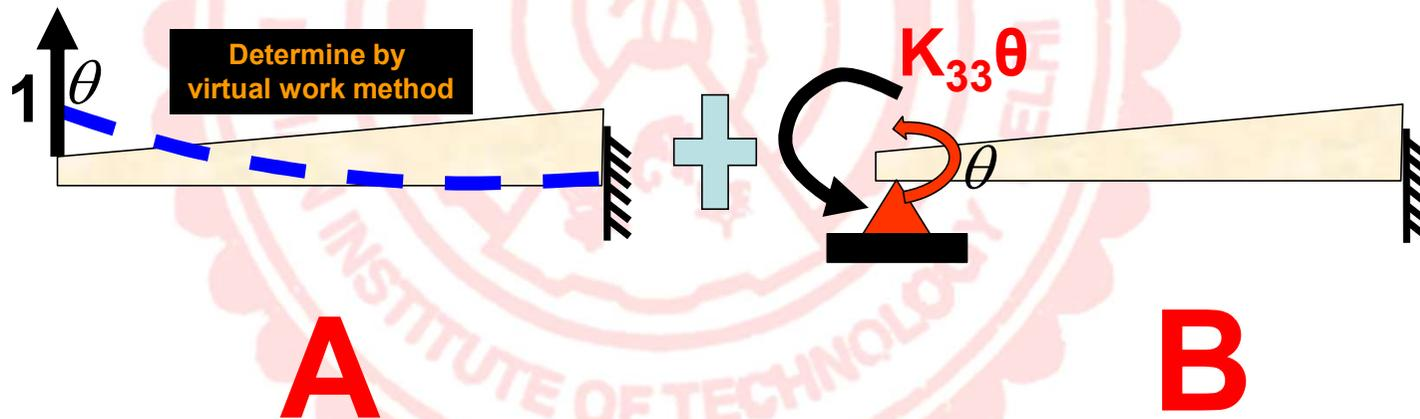
Choose multipliers such that the net angle of rotation on the left end of the beam is **ZERO**
