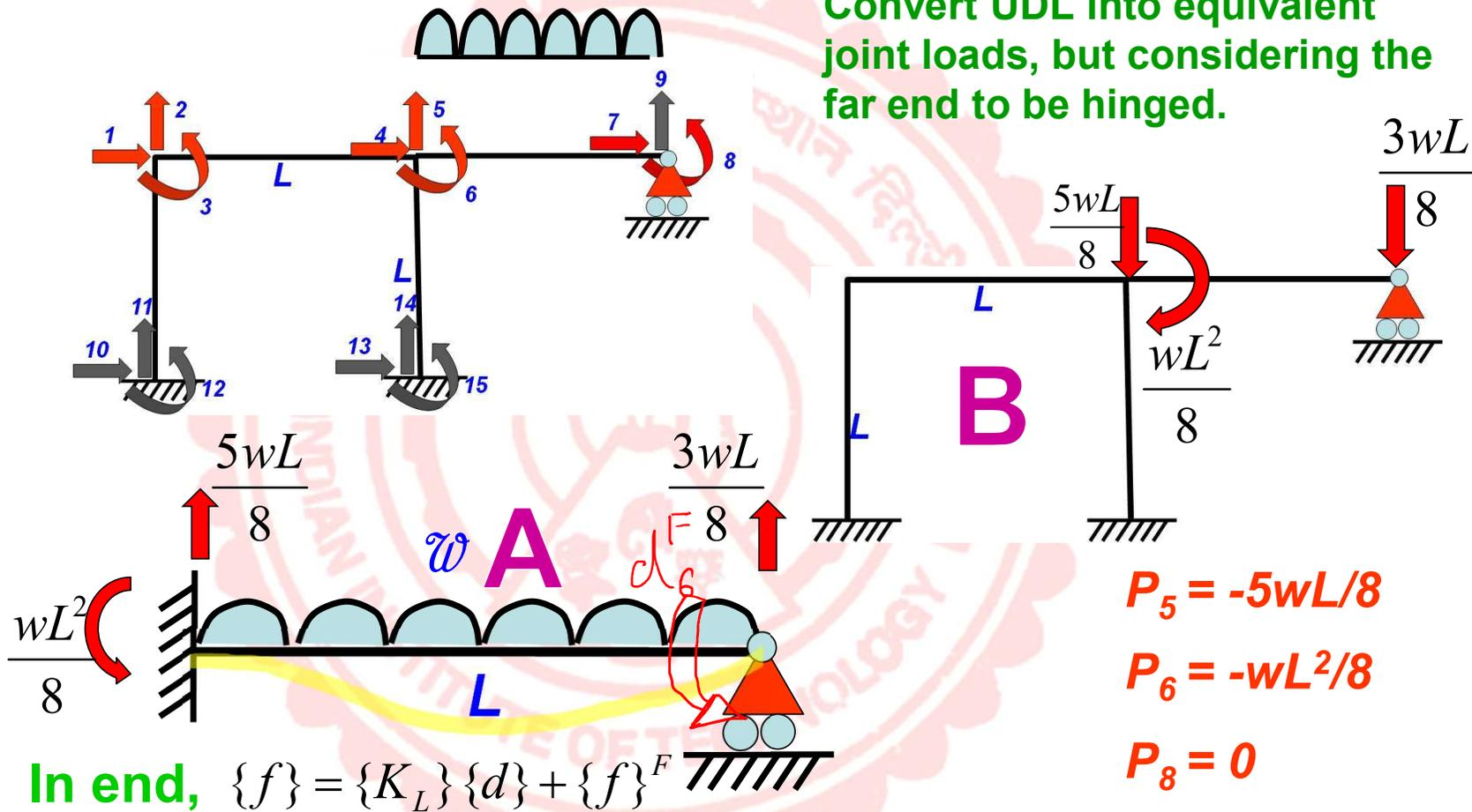
**Caution:** Displacement correction needed in end.  $d^f$  to be added to the displacement from the output
