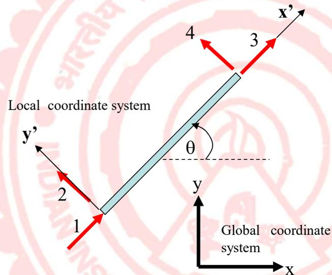
$$\begin{Bmatrix} f_1 \\ f_2 \\ f_3 \\ f_4 \end{Bmatrix} = \begin{bmatrix} \frac{EA}{L} & 0 & -\frac{EA}{L} & 0 \\ 0 & 0 & 0 & 0 \\ -\frac{EA}{L} & 0 & \frac{EA}{L} & 0 \\ 0 & 0 & 0 & 0 \end{bmatrix} \begin{Bmatrix} d_1 \\ d_2 \\ d_3 \\ d_4 \end{Bmatrix}$$
