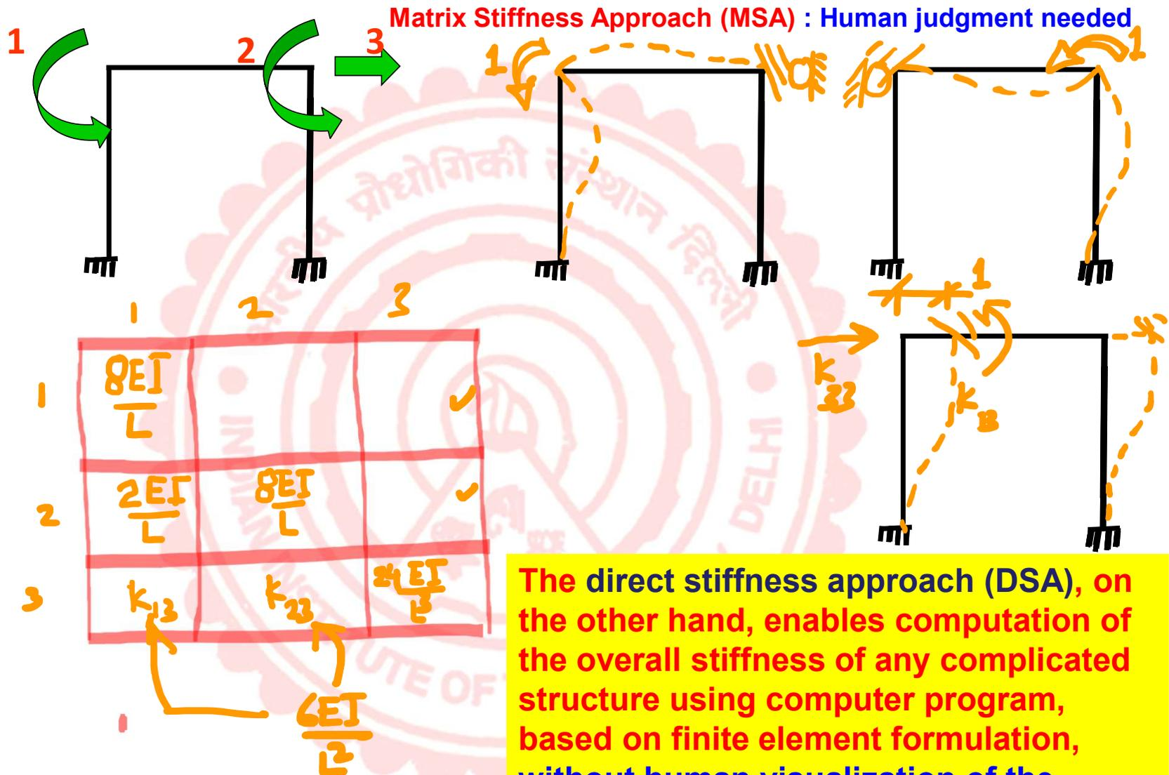
The direct stiffness approach (DSA), on the other hand, enables computation of the overall stiffness of any complicated structure using computer program, based on finite element formulation, without human visualization of the overall structure.
