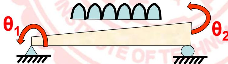
*Both rotations can be obtained using the principle of virtual work*
