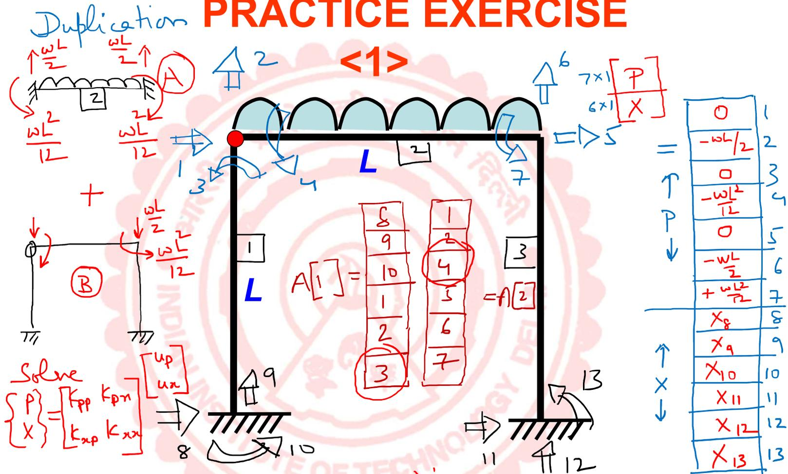
Solve  $\begin{Bmatrix} P \\ X \end{Bmatrix} = \begin{bmatrix} k_{pp} & k_{pn} \\ k_{np} & k_{nn} \end{bmatrix} \begin{Bmatrix} u_p \\ u_n \end{Bmatrix}$
