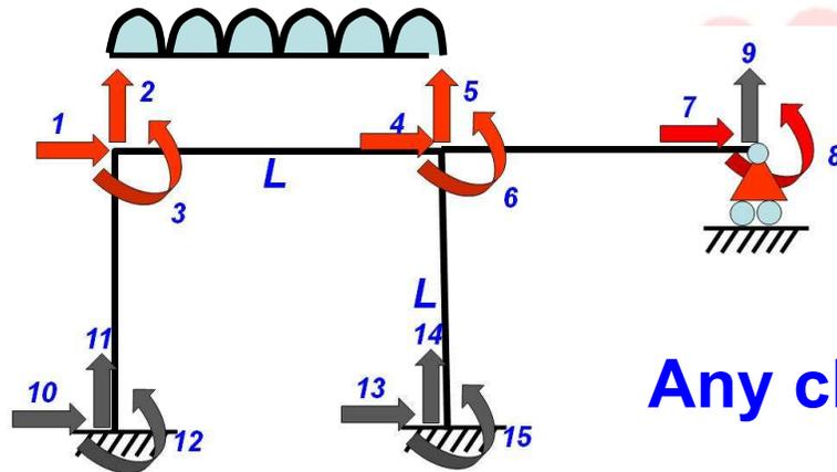
Convert the UDL into equivalent joint loads
