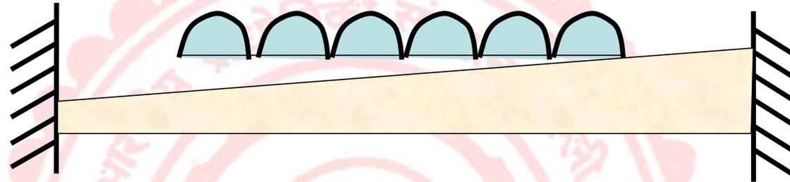
Release the restraints and convert the structure into a determinate system
