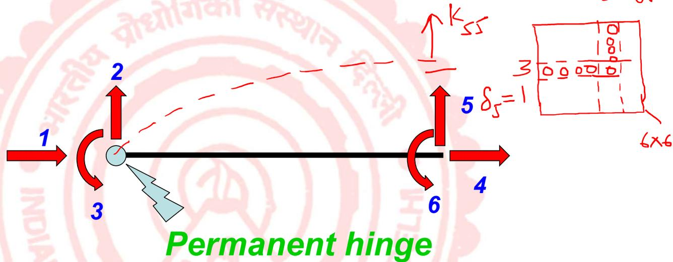
*This boundary condition is not to be altered while deriving the member stiffness matrix*
