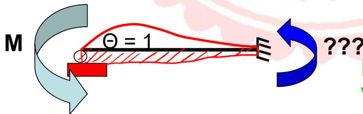
Being indeterminate, principle of Virtual Work cannot be applied
