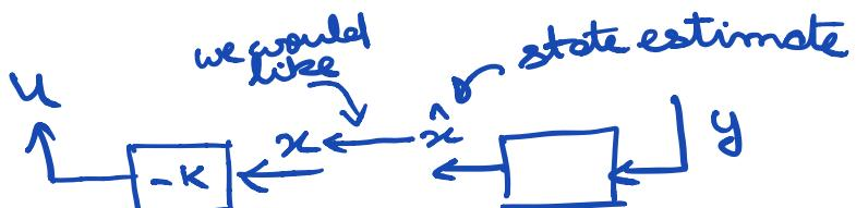
$$\begin{aligned} \text{eqn: } u &= -Kx \\ &\quad + k_x r \\ &\text{reference } \rightarrow \end{aligned}$$
