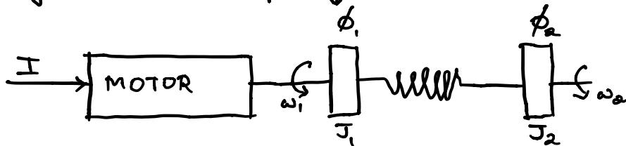
This system can represent a motor with a flexible shaft that drives a load. Assuming that the motor delivers a torque that is proportional to the current  $I$ , the dynamics of the system can be described by the equations,
