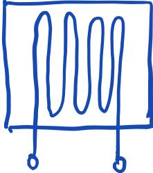
strain in this direction measured
