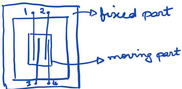
1, 2, 3, 4 → conductors under strain
