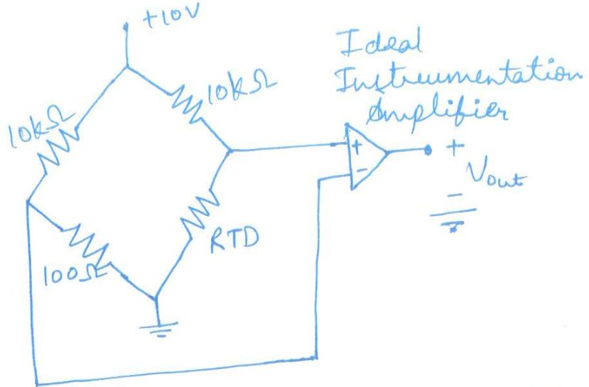
The differential gain of instrumentation amplifier to achieve a voltage sensitivity of  $10\text{mV}/^\circ\text{C}$  at  $0^\circ\text{C}$  should be approximately?
