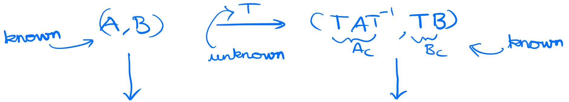
$W_c = [B \quad AB \quad \dots \quad A^{n-1}B]$
