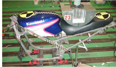
Fig.5 Compression test of a seat.
