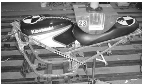
Fig.5 Compression test of a seat.
