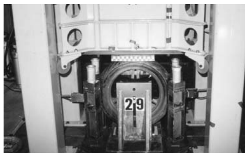
Fig.4 Drop test of a front wheel.
