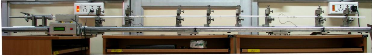
Figure 4: SHPB setup using PTFE bars
