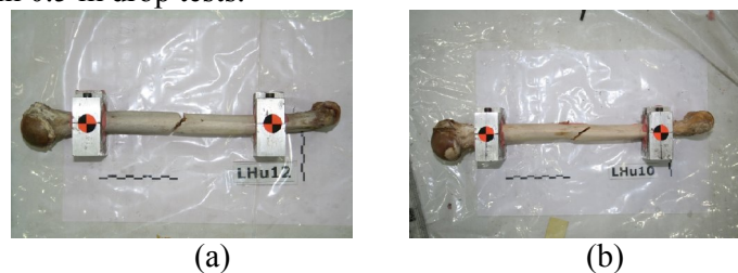
Figure 5 Fracture types observed in experiments. Each black rectangle is 20 mm.
