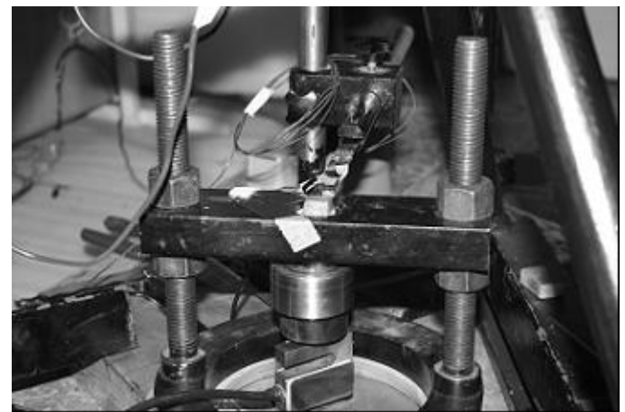
Figure 2. Impact Gun test set-up, launcher is not shown in the picture
