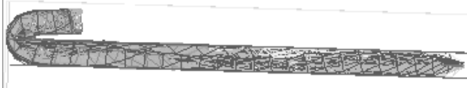
Figure. 4 Side view of airbag mesh showing folded top portion of airbag mesh.
