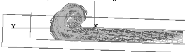
Figure. 5 Side view of airbag mesh showing second fold of top portion of airbag mesh.
