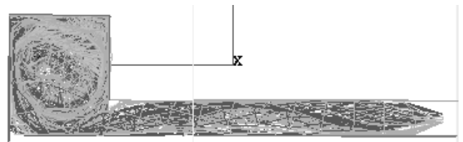
Figure. 8 Side view of airbag mesh showing squeezed top folded portion.
