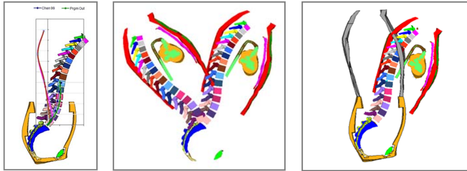
Figure 2 –(L-R) (a) 30° flexed posture of FE-HBM upper extremity about the lumbo sacral joint (Adapted from Marathe et. al., 2010) (b) Transformed mesh of upper extremity with change in spine posture. (c) Flexed posture of upper extremity along with initial mesh of pelvis flesh.
