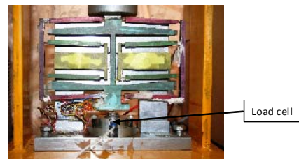
Figure 4. Load cell inside the specimen subassembly.
