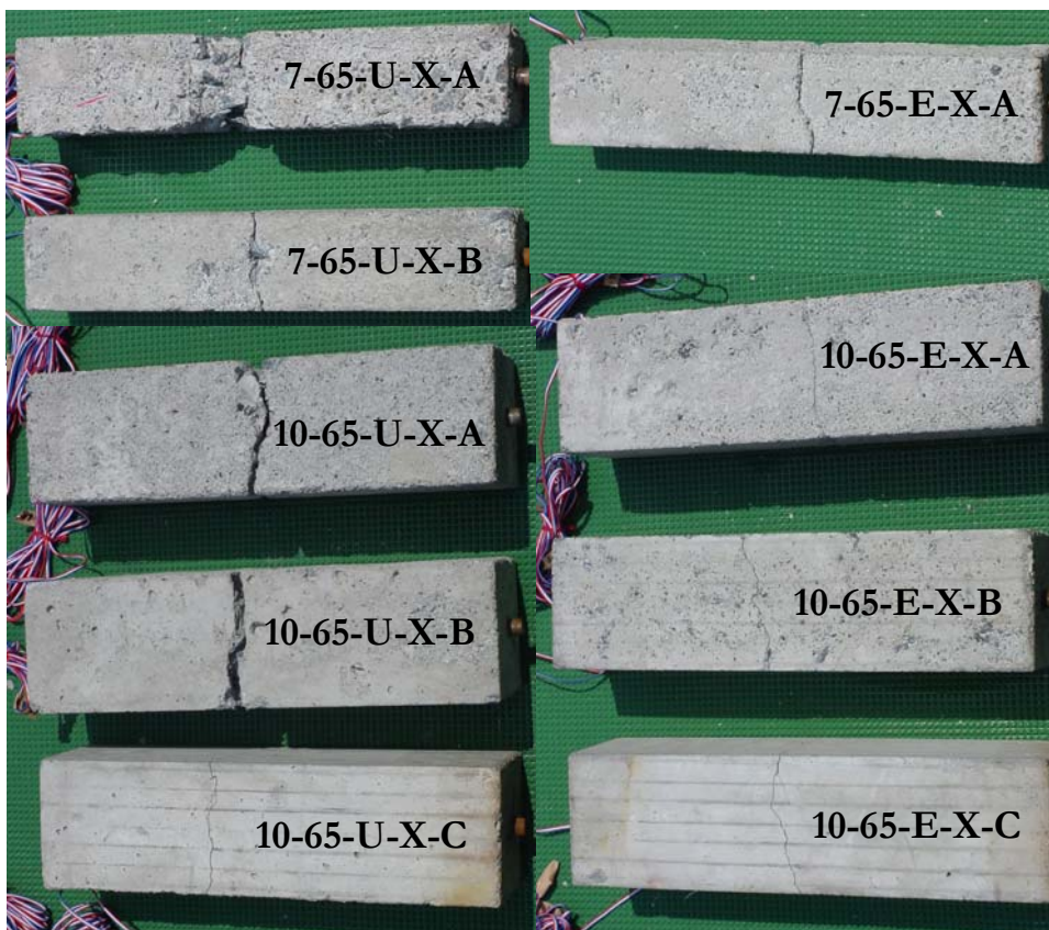
Fig. 3.22: Cracked specimens after freeze-thaw deterioration
