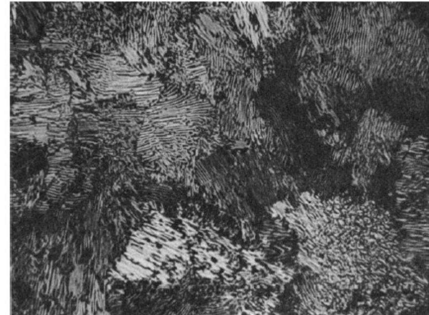
Image of pearlite with dark field illumination
