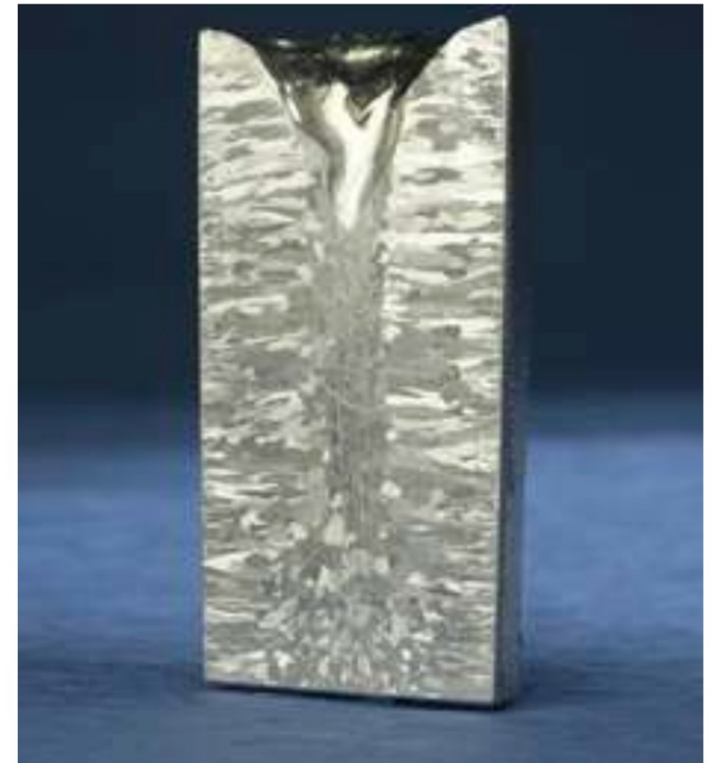
Section of cast ingot illustrating the microstructure
