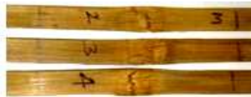
Fig.10B. Tensile failure mode of single laminas of nodal.
