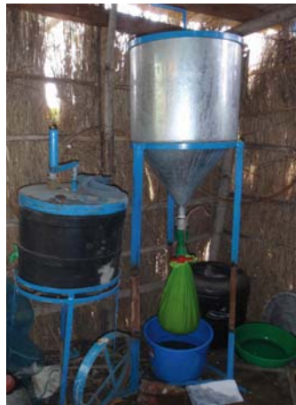
Figure 21. Manually operated reactor for recovery of struvite (Source: Eawag)
