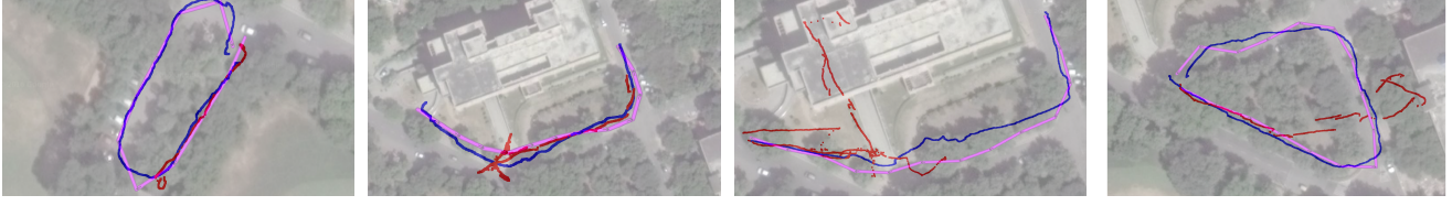
Figure 5. Comparison of trajectories obtained for egocentric videos. In each of these images the trajectories obtained by our method are marked in blue, while those attained by LSD-SLAM are marked in red. Due to the lack of any standardized datasets with ground truth poses for egocentric videos, the accuracy of the trajectories is demonstrated by overlaying them on GPS data (pink). It should be noted that the LSD-SLAM trajectories shown here are the ones obtained just before the algorithm crashed. The frequent crossed trajectories in LSD-SLAM results is due to noisy 3D estimates maintained by the algorithm which often leads to false matches
