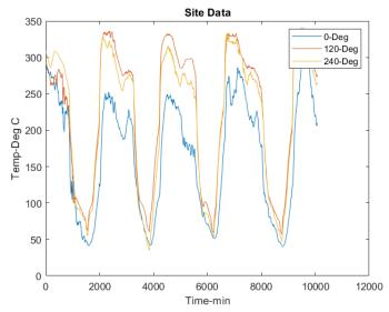
The minute-wise data are easily extracted and plotted and visually compared using Matlab. Further the Data obtained has to be filtered and studied. Deg, Deg1 & Deg 2 are Thermocouple Probes.
