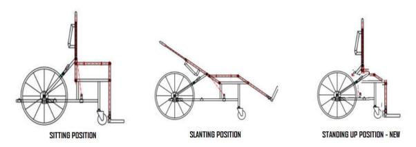
In general, wheel chair are primarily designed for sitting position and in some recent developments wheelchairs are provided with slanting mechanisms. This facilitates users comfortable horizontal laying position.
