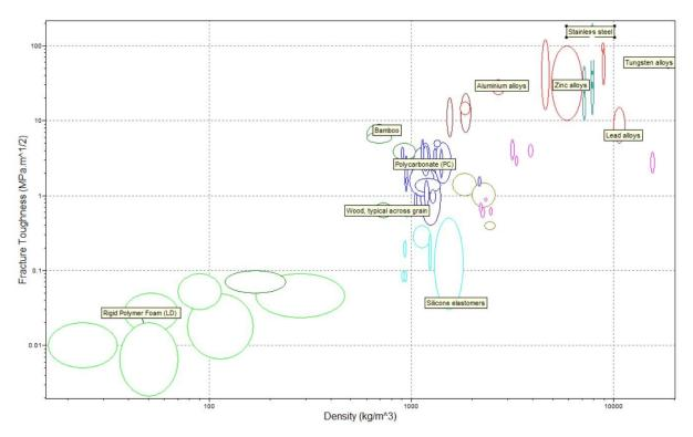
Criteria for Stage 3: Fracture Toughness determines the resistance of Crack propagation once crack has been initiated in the structure. Lower the value brittle is the material, with little load or damage initiation the metal will shatter immediately. On the same front, with higher value of Fracture Toughness, material will deform more & more before tearing.
