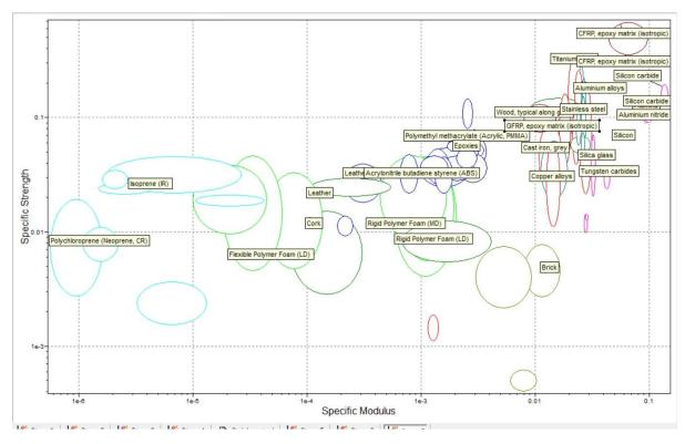
Criteria for Stage 6: The ratio of Strength of the Material to its density is the defined as specific strength of the material. This formulation is done by using advanced feature of CES tool. Similarly, the ratio of Young's modulus to it's respective density is called as Specific modulus of the material. Aluminium shares the capabilities similar to stainless steel. Less weight with more strength is most preferred. As so, aluminium alloys fits best in the lot.
