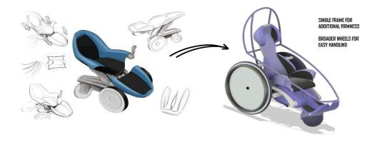
With the help of advanced CAD softwares available, many concepts were developed and investigated for its advantages and disadvantages. Stating the primary agenda of making frame of wheel chair lighter and stronger, CES EDU PACK has been used.
