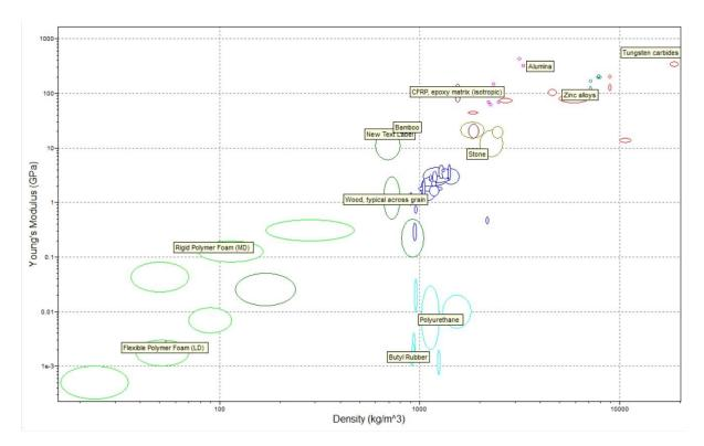
Criteria for Stage 2: Young's Modulus determines the stiffness or sag ability of Material of construction. Dut of shortlisted materials ascending order of materials in accordance with higher rankings are sorted.
