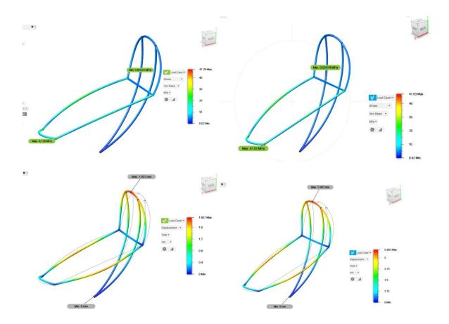
From static analysis of Chasis with the nominal propable maximum average load steel and aluminium structures where compared. The factor of safety wasa almost at par however, aluminium deforms more than the steel, but with in the permissible limits. To attain cushioning effect of the seat, and to provide comfort and support a Laser Sintering approach using TPU materials shall be selected for its flexibility and strength.
