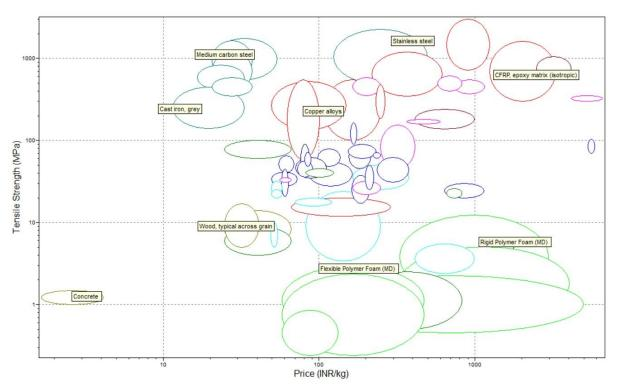
Criteria for Stage 4: Cheaper material is always preferred in the industry and cheaper material with higher strength is added advantage. Based on the priority criteria we have the shortlisted remains almost same.
