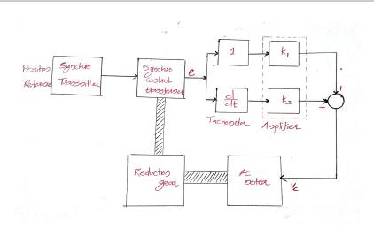
Figure: AC Position control system
