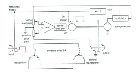
Figure: AC Position control system layout
