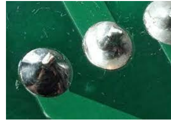
A good solder joint
