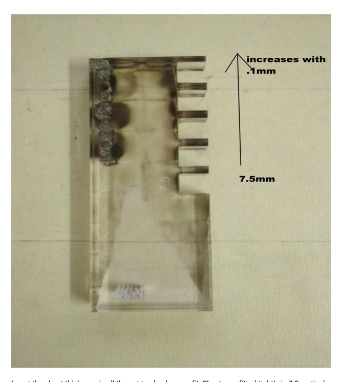
Insert the sheet thickness in all the cut to check press fit. Sheet was fitted tightly in 7.9 vertical.
