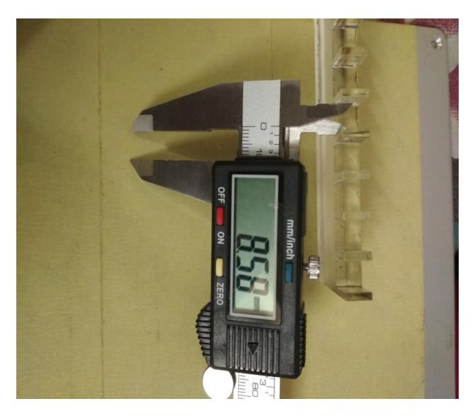
It means that the laser cut  $\,$  more than the given value. For press fit I tested with another comb having dimension 7.9 to 7.5  $\,$
