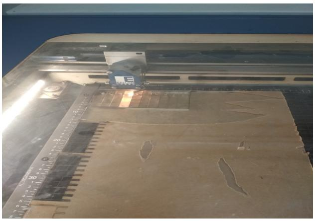
For this speed 5%, power 100%, frequency 100%. Didn't cut in single pass so again pressed 'GO' to cut.
