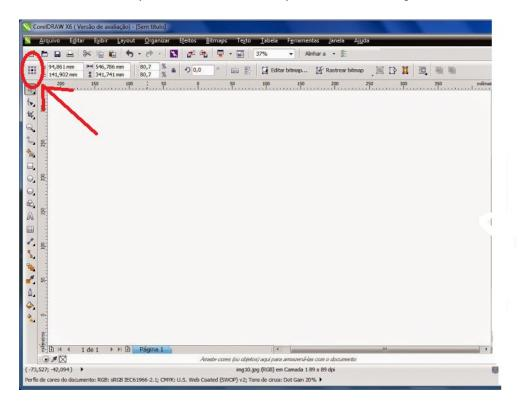
4. Give x distance in positive and y distance in negative according to the length and width of sheet on which the design is going to cut.
