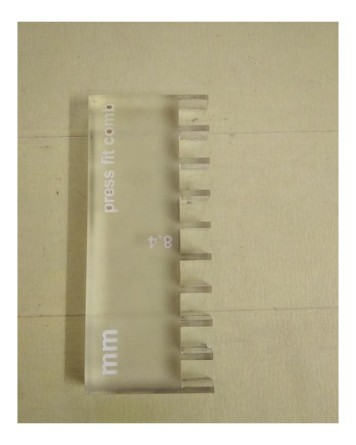
8.4 mm was given for vertical cut .This dimension is same as the thickness of sheet. But the thickness of sheet didn't fit tightly in the 8.4 vertical cut section.
