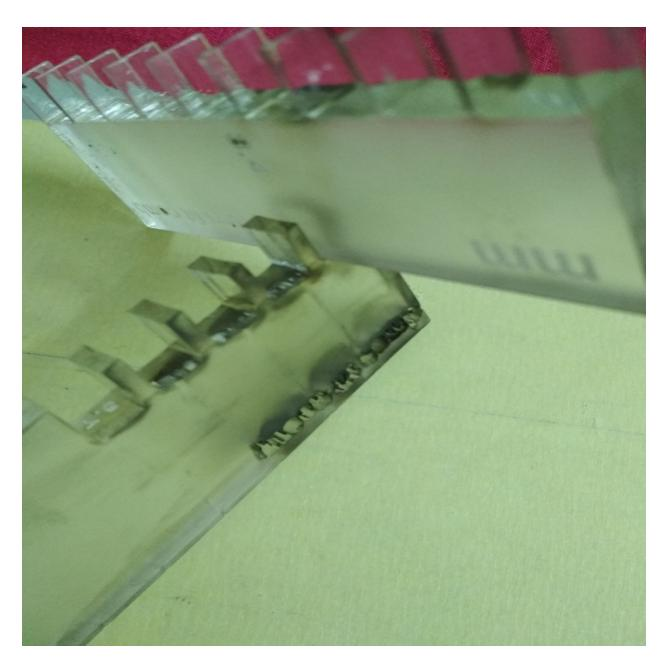
Measured the 7.9 cut, it was showing 8.35 in digital caliper. The difference between the cut sheet and original dimension was .45mm or approx .5mm.This is known as kerf. Each side the kerf was .25mm.
