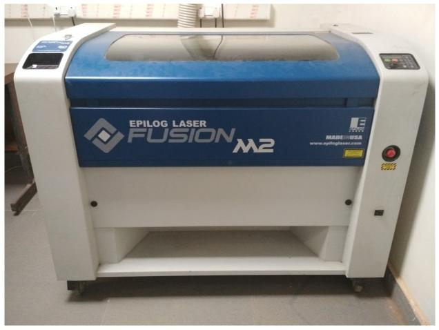
This machine uses CO2 gas for production of laser (CO2 laser is 10.6 micrometer in wavelength) and uses maximum 60 watt power. And with the help of gauge we fix the distance between the material and nozzle. The gauge height is 2".
