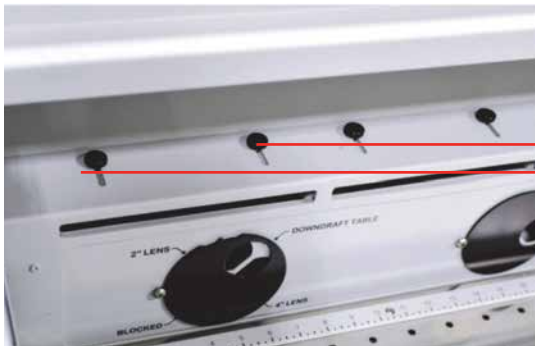
Two thumb screws to adjust air flow for each section.
