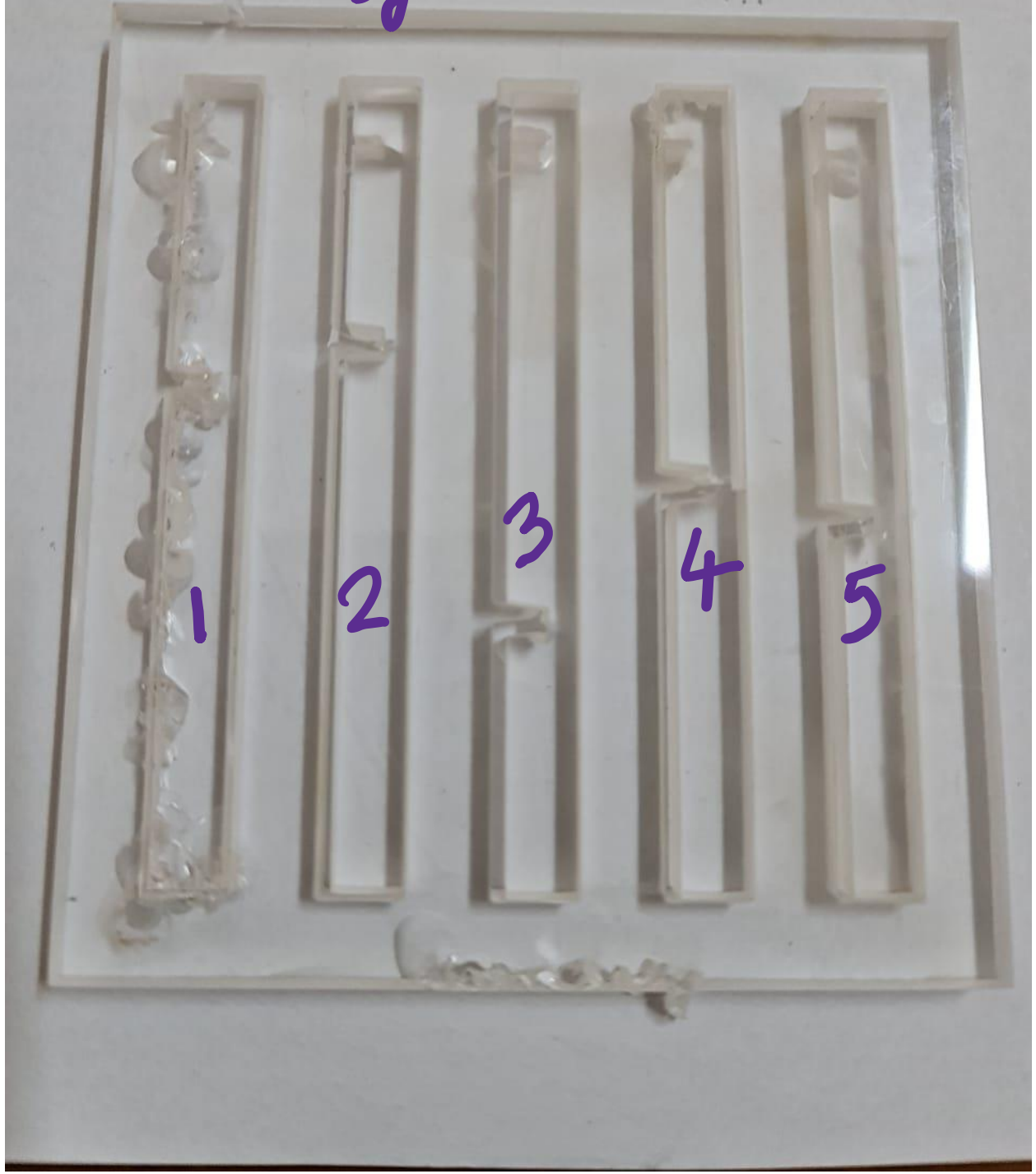
Brittle material acrylic not cut properly.
