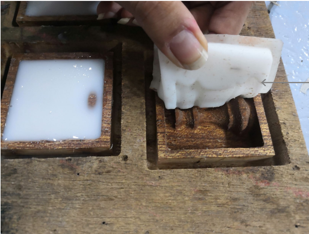
← removing the mould from the cast
