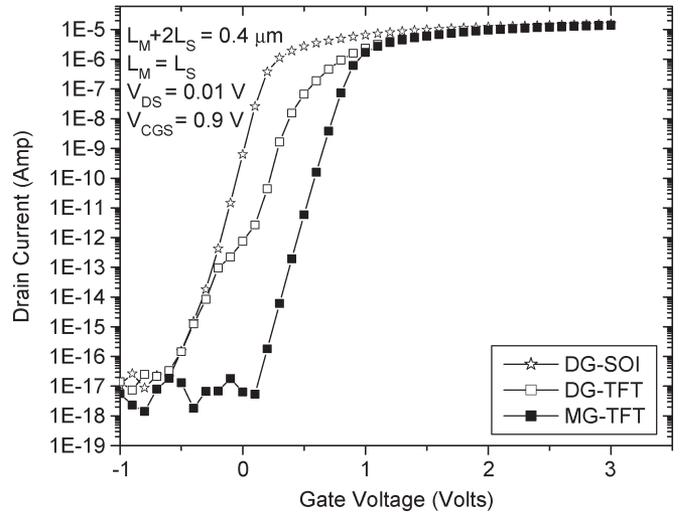
Fig. 3. Transfer characteristics of MG-TFT, DG-TFT, and DG-SOI structures.
