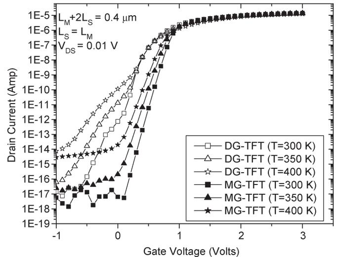
Fig. 8. Transfer characteristics of MG-TFT and DG-TFT for different temperatures.
