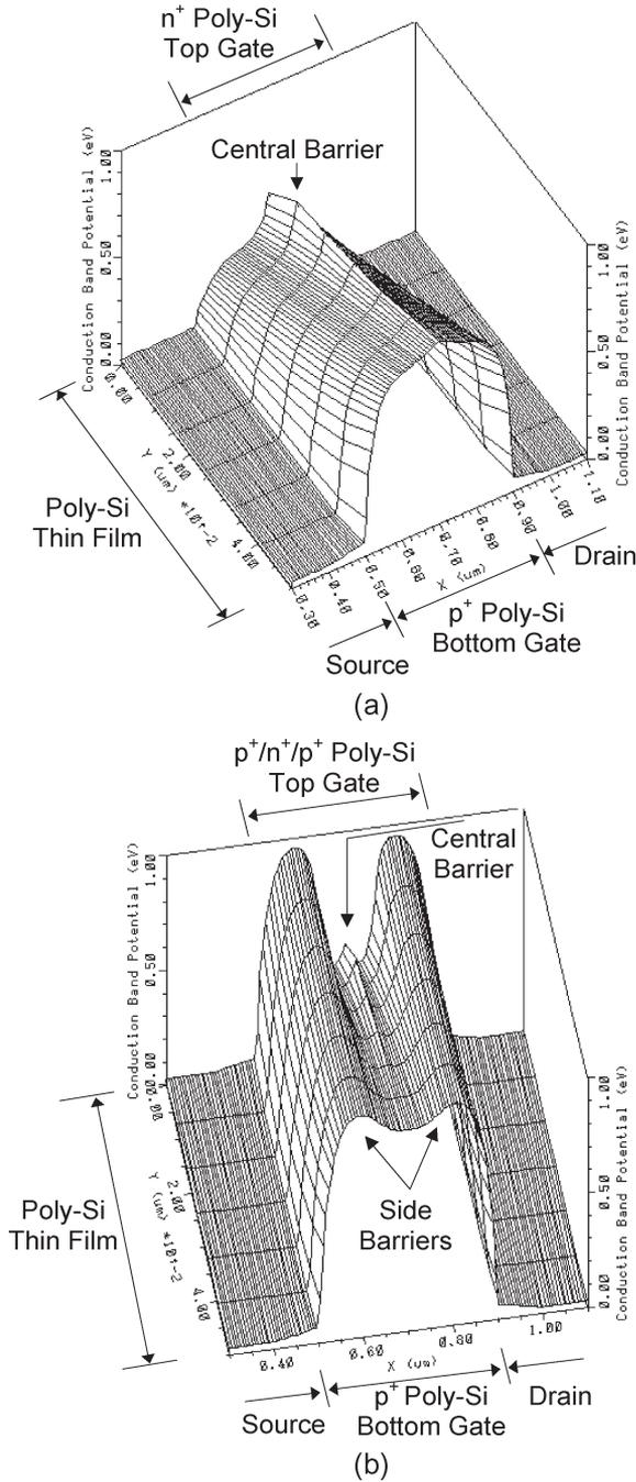
Fig. 2. Conduction-band potential distribution for (a) DG-TFT and (b) MG-TFT structures for  $V_{GS} = 0$  V and  $V_{DS} = 0$  V.
