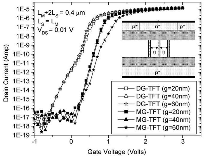
Fig. 12. Transfer characteristics of MG-TFT and DG-TFT for three GBs in the main channel.
