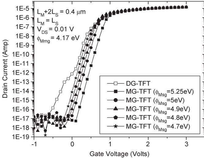
Fig. 5. Transfer characteristic of the MG-TFT structure for different work functions of the side gates.
