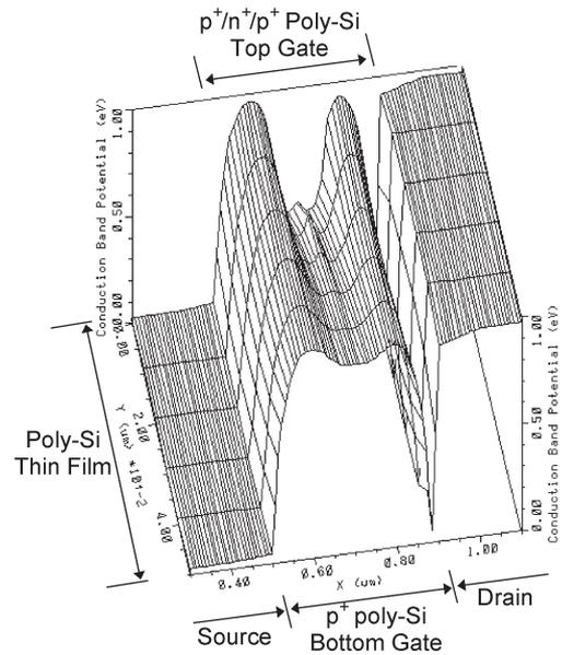
Fig. 4. Conduction-band potential distribution for the MG-TFT structure with  $V_{GS} = 0$  V and  $V_{DS} = 1$  V conditions.
