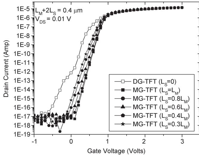
Fig. 9. Transfer characteristics of MG-TFT for different side-gate lengths.  $L_M$  and  $L_S$  are the main- and side-gate lengths, respectively. The channel length ( $L = 2L_S + L_M$ ) is fixed at  $0.4 \mu\text{m}$ .
