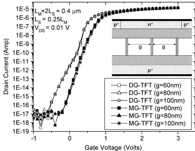
Fig. 14. Transfer characteristics of MG-TFT and DG-TFT for three GBs in the channel for small side-gate length ( $L_S = 0.25L_M$ ).
