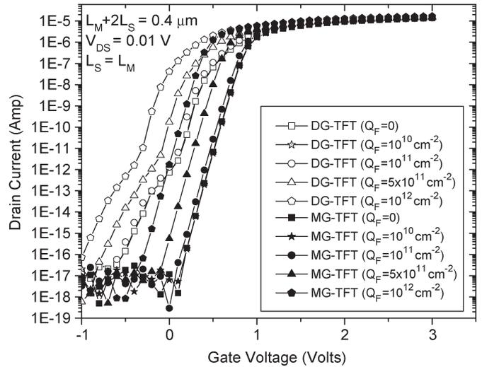
Fig. 11. Transfer characteristics of MG-TFT and DG-TFT for different fixed charges at the interface between the top/bottom gate and poly-Si thin film.
