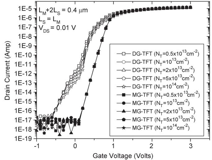
Fig. 7. Transfer characteristics of MG-TFT and DG-TFT for different trap densities. The values of central-barrier height at the center of the GB for trap densities  $5 \times 10^{12}$ ,  $10^{13}$ ,  $2 \times 10^{13}$ ,  $5 \times 10^{13}$ , and  $10^{14} \text{ cm}^{-2}$  are 0.65, 0.67, 0.7, 0.72, and 0.74 eV, respectively, for  $V_{GS} = 0 \text{ V}$  and  $V_{DS} = 0 \text{ V}$ .
