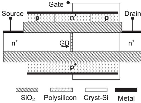
Fig. 1. Cross-sectional view of the asymmetrical MG-TFT.
