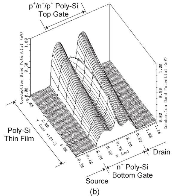
Fig. 15. Conduction-band potential distribution for (a) SDG-TFT and (b) SMG-TFT structures for  $V_{GS} = 0$  V and  $V_{DS} = 0$  V. The SMG-TFT structure is a multiple-gate structure made on an SDG-TFT.
