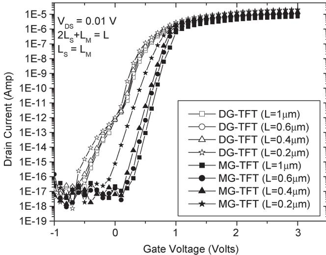
Fig. 6. Transfer characteristics of MG-TFT and DG-TFT for different channel lengths.
