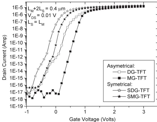
Fig. 16. Transfer characteristics of DG-TFT, MG-TFT, SDG-TFT, and SMG-TFT structures. The DG-TFT and MG-TFT are asymmetrical structures, while the SDG-TFT and SMG-TFT are symmetrical structures under the main gate.
