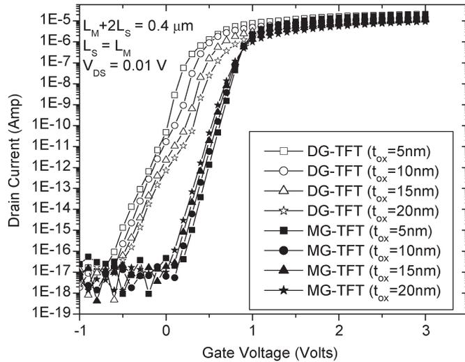
Fig. 10. Transfer characteristics of MG-TFT and DG-TFT for different gate-oxide thicknesses.
