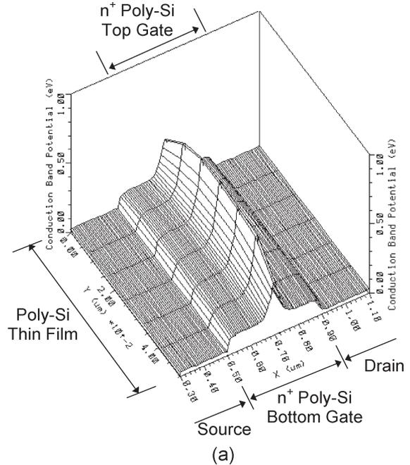
Fig. 13. Conduction-band potential distribution of the MG-TFT structure with three GBs in the channel ( $g = 60$  nm) for  $V_{GS} = 0.5$  V and  $V_{DS} = 0.01$  V.
