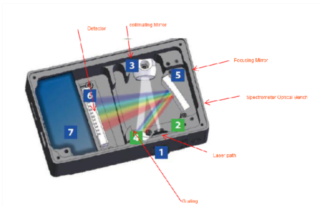
Figure 10.4: Schematic of the inside of the Raman spectrometer that you are using. The wavelength of the laser is 532 nm and the detector is a CCD detector having a linear array of 3648 pixels. The position labeled 4 corresponds to that of a monochromator with the grating of 1200 grooves/mm.
